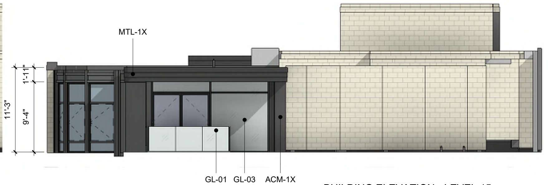
BUILDING ELEVATION - LEVEL 15 SOUTH - CAPITOL SIDE 1/8" = 1'-0"
