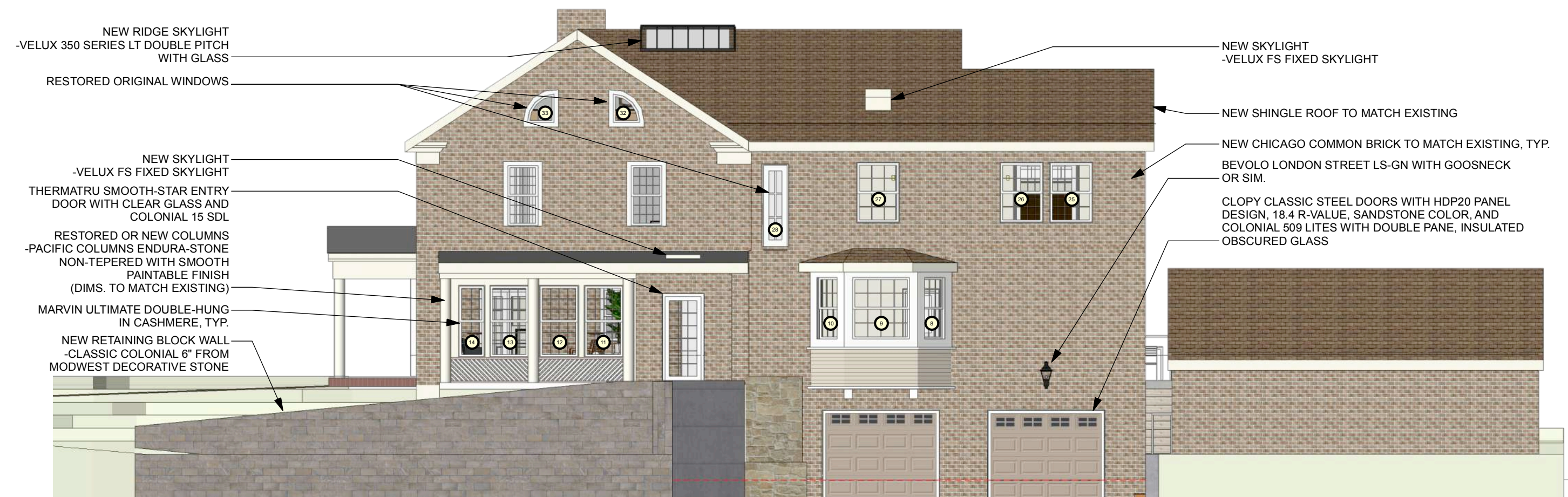
18 PROPOSED WEST ELEVATION Scale: 1/8" = 1'-0"
