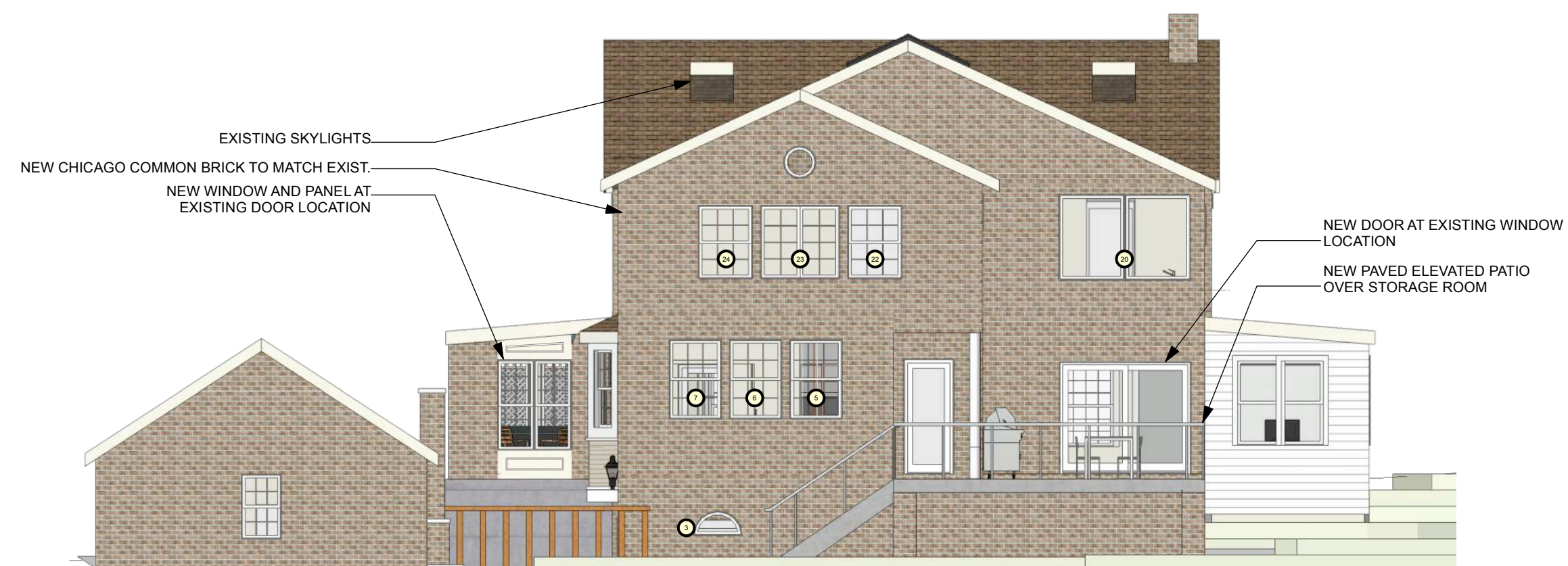
20 PROPOSED SOUTH ELEVATION Scale: 1/8" = 1'-0"
