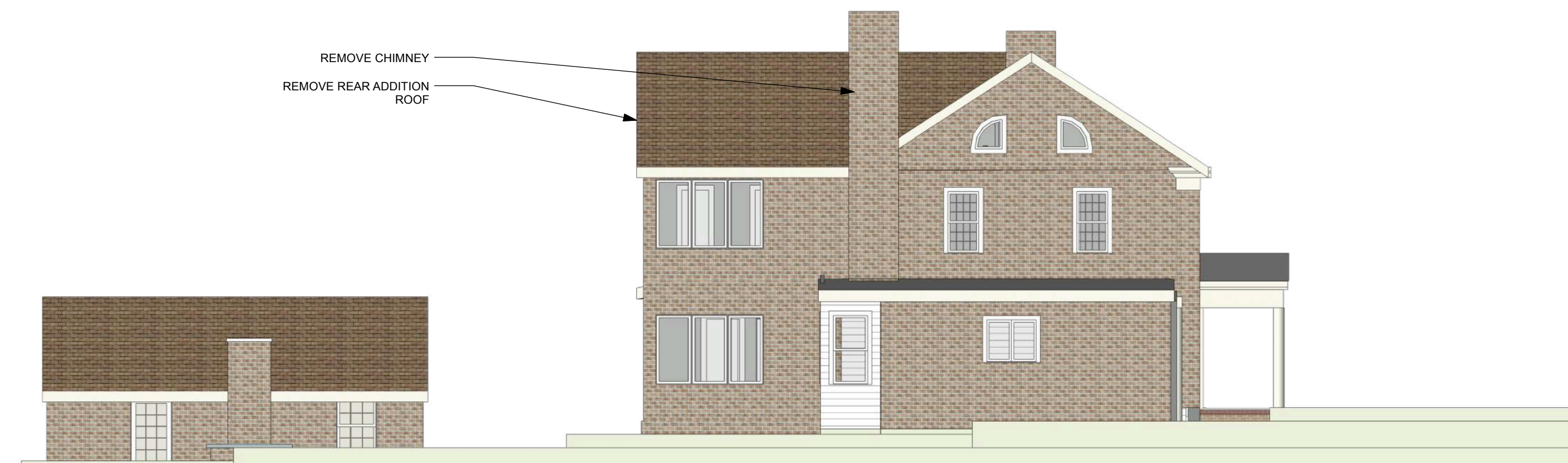
EXISTING EAST FACADE DETAIL - CHIMNEY AND CAP TO BE RESTORED, QUARTER ROUND WINDOWS TO BE REHABILITATED, AND HVAC CONDUIT TO BE ELIMINATED
