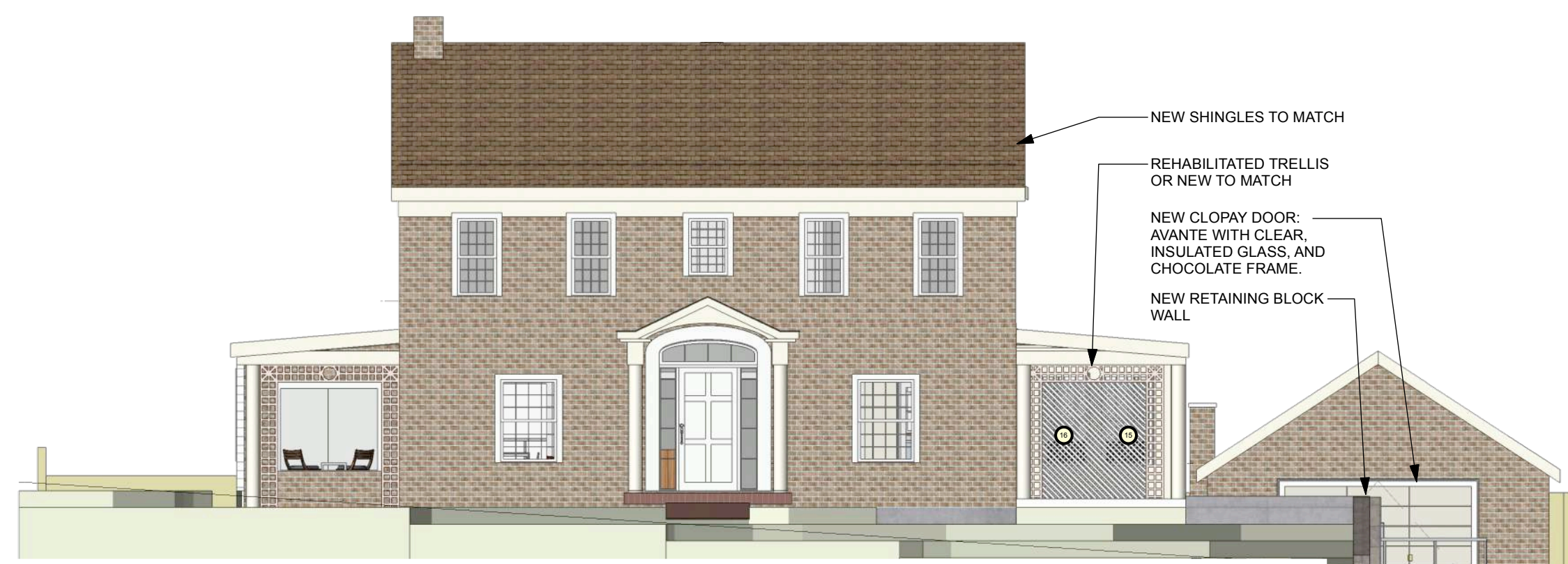
16 PROPOSED NORTH ELEVATION Scale: 1/8" = 1'-0"
