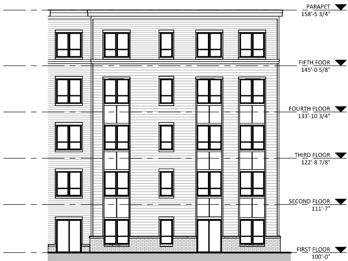
2 CITY ELEVATION - COURTYARD NORTHWEST 3/32" = 1'-0"
