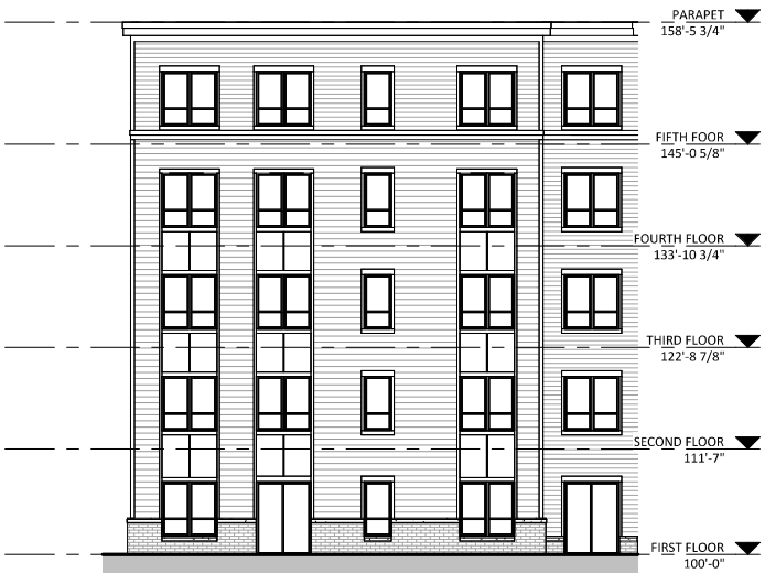
3 CITY ELEVATION - COURTYARD SOUTHEAST 3/32" = 1'-0"
