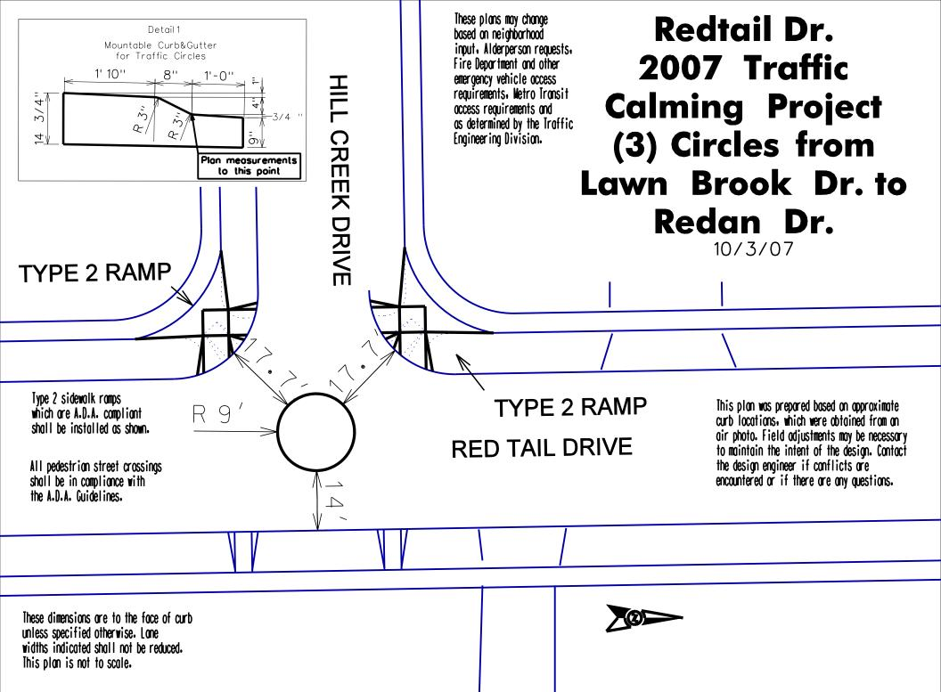
Type 2 sidewalk ramps which are A.D.A. compliant shall be installed as shown.
