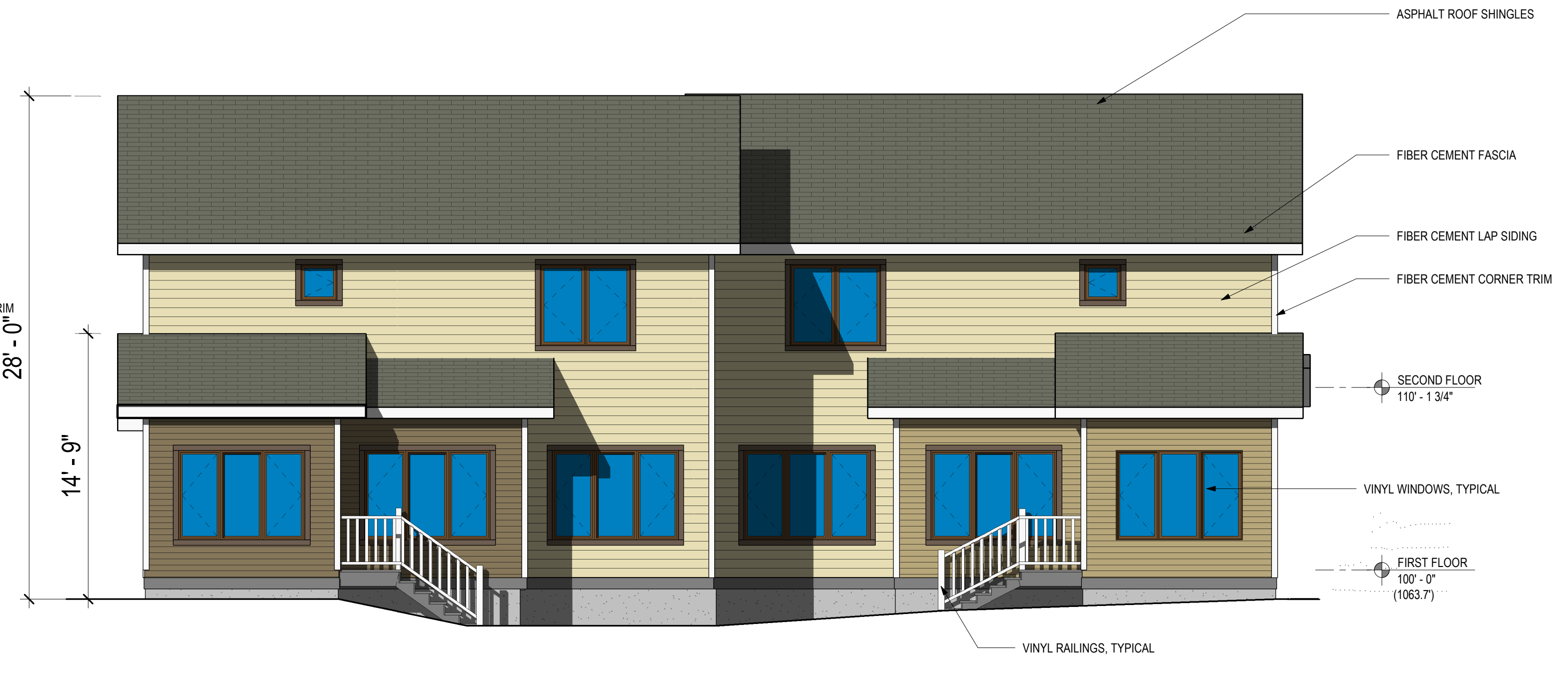
3 SOUTH ELEVATION - DUPLEX (A)
