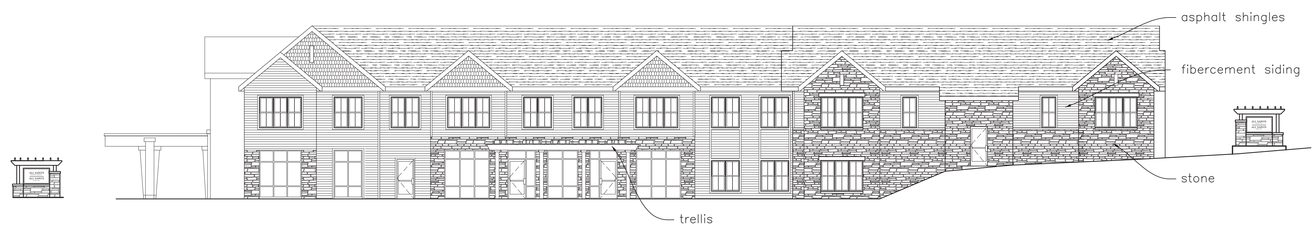
4 SOUTH ELEVATION OF CBRF AT DRIVE LANE
