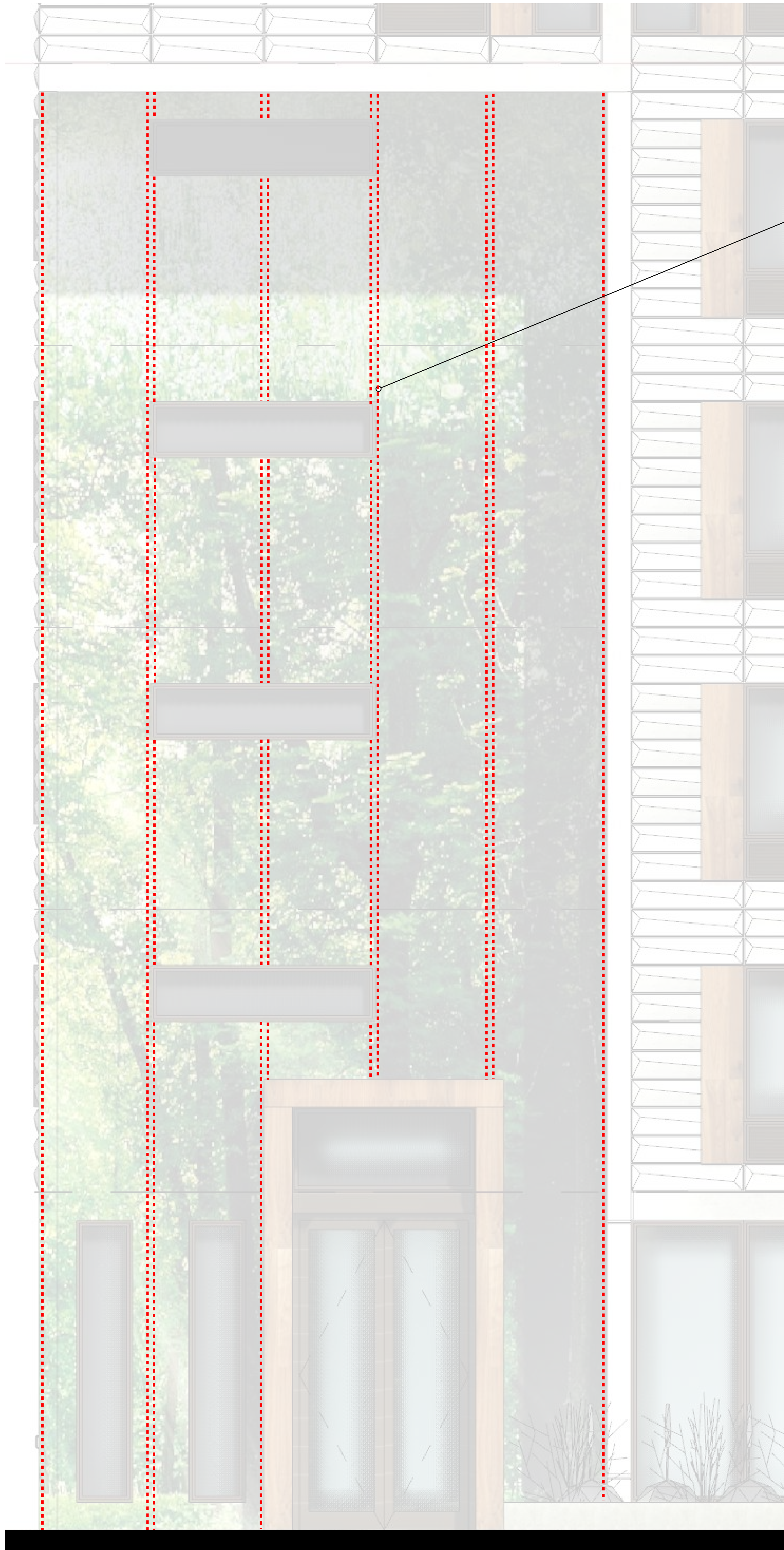
2 North Curtain wall LED light locations
