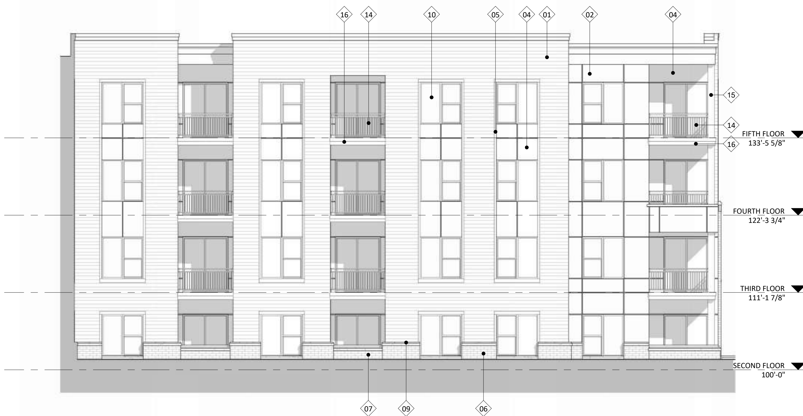
2 ELEVATION - COURTYARD NORTH AC202 1/8" = 1'-0"
