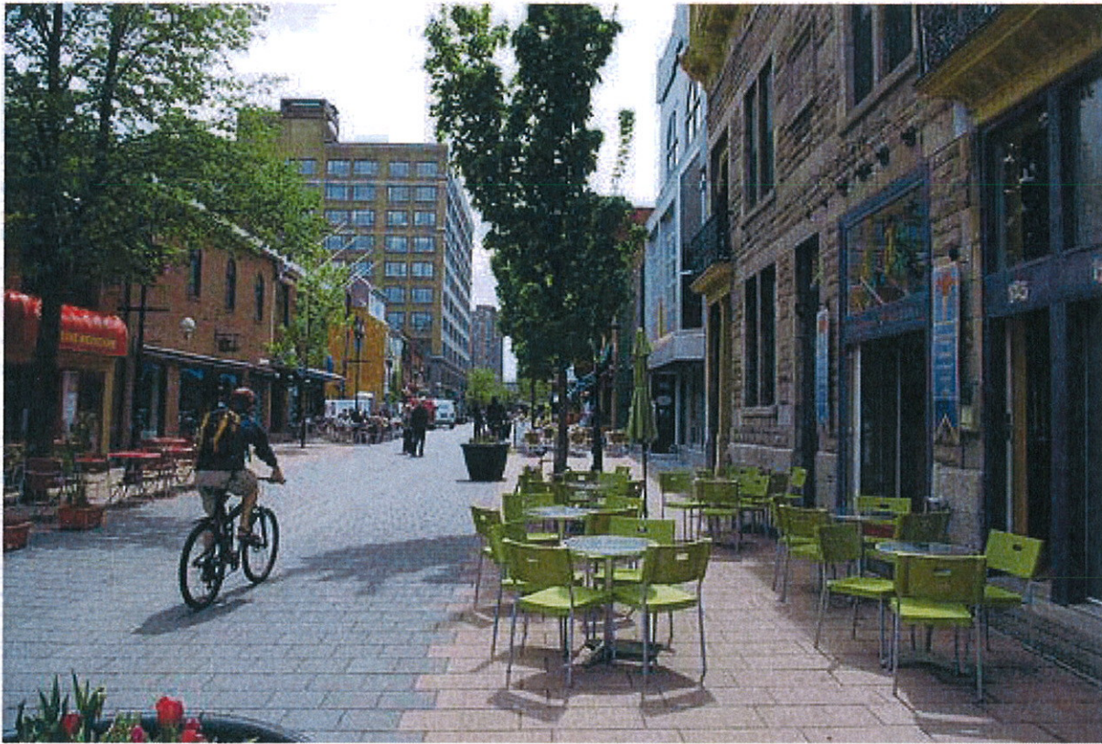
A sidewalk level street with pedestrian style paving, no traffic lines and pedestrian scale landscaping.
