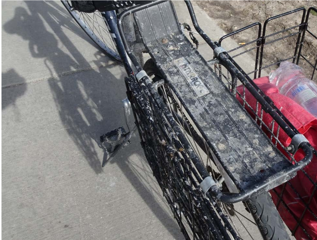
Salt coating from brine slush on SW Path during 2015-16 "pilot program"
