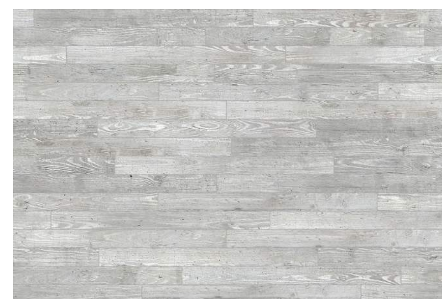
BOARD FORMED CONCRETE
