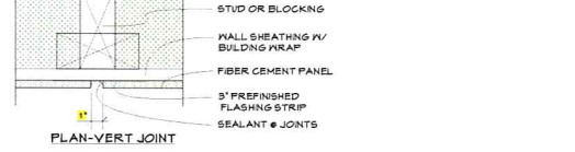
5 PANEL JOINT DETAIL A-6 Scale: 3/4" = 1'-0"
