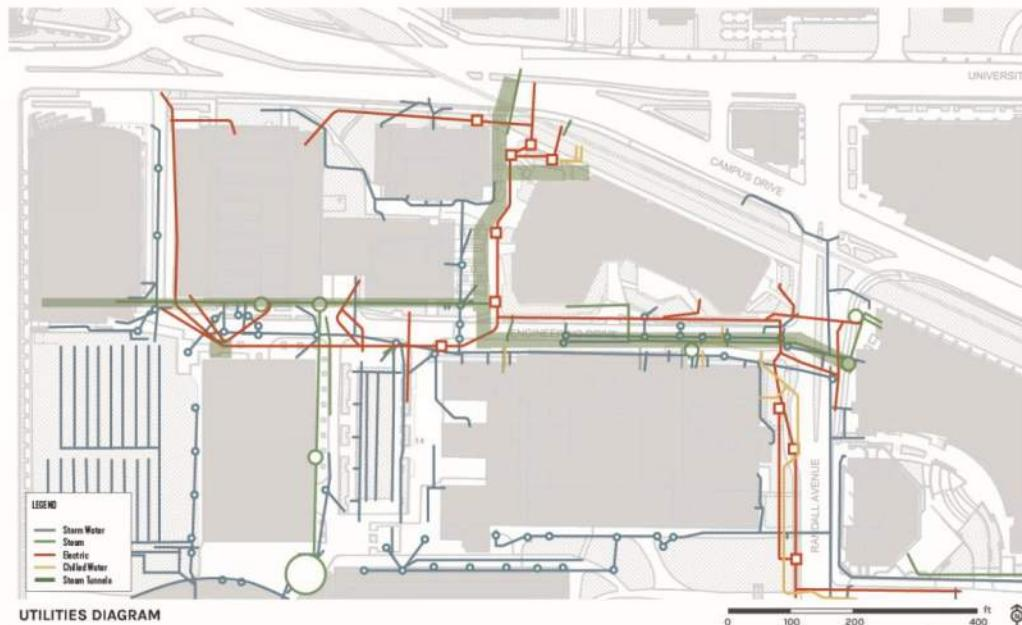
**Note:** The steam and chilled water lines currently east of the parking structure are radial feeds serving the Athletic Complex south of this area. They can be relocated but will need to maintain services.
