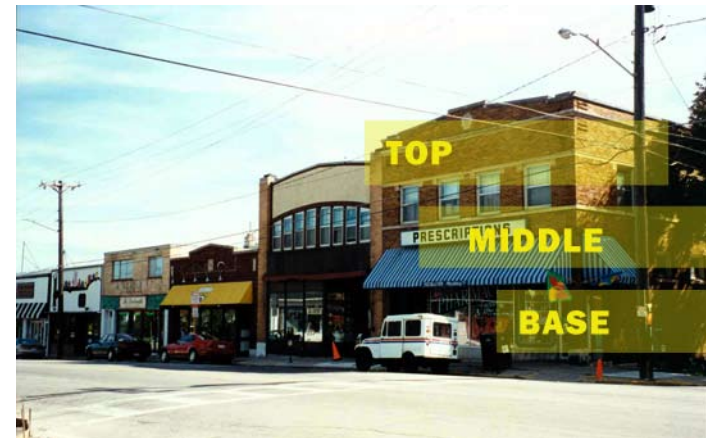
Figure J-2: Expression of Base, Middle and Top in Existing Monroe Street Buildings
