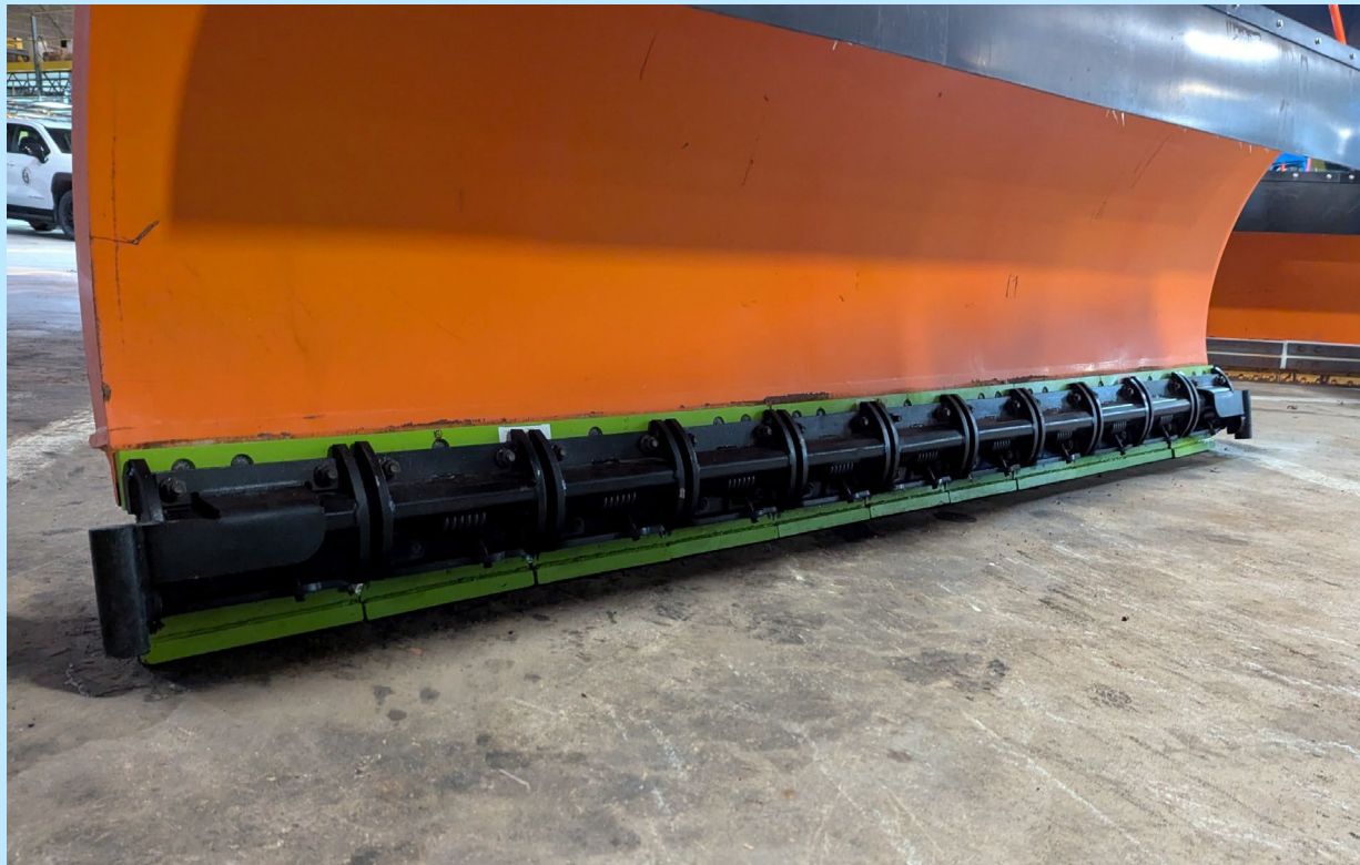
Piloting new style of plow blade that may conform with the road surface better
