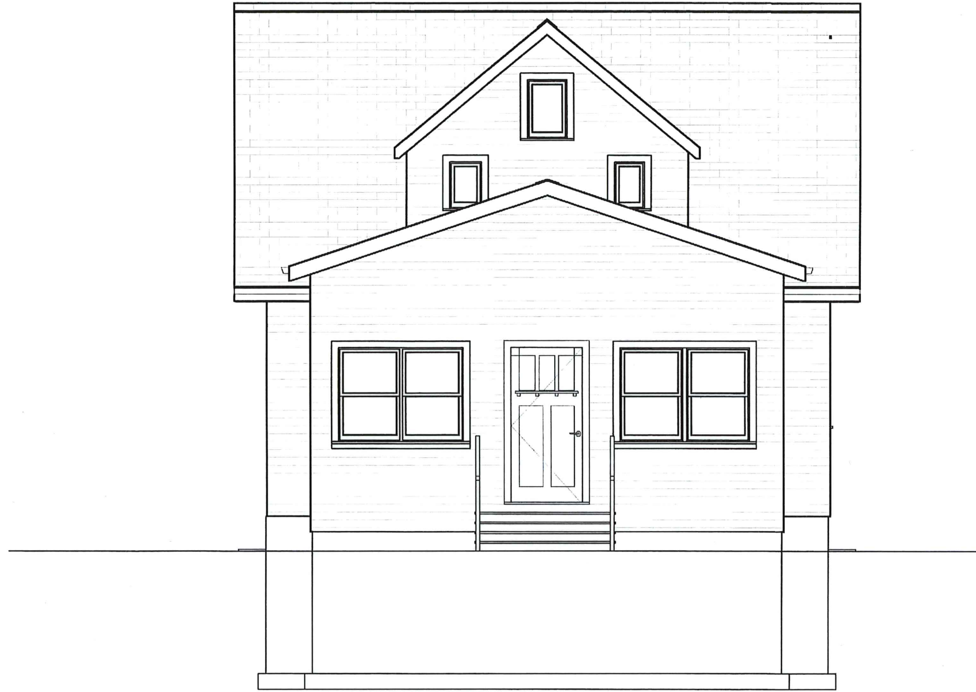
Front (North) Elevation of Existing and with Proposed Rear Additions Does Not Change 1/4" = 1'
