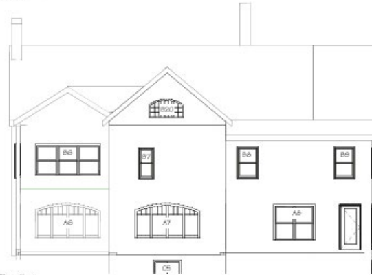
① Proposed East Elevation 1/8" = 1'-0"
