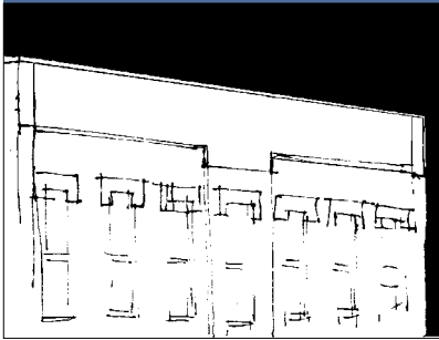
Existing building with missing cornice.
