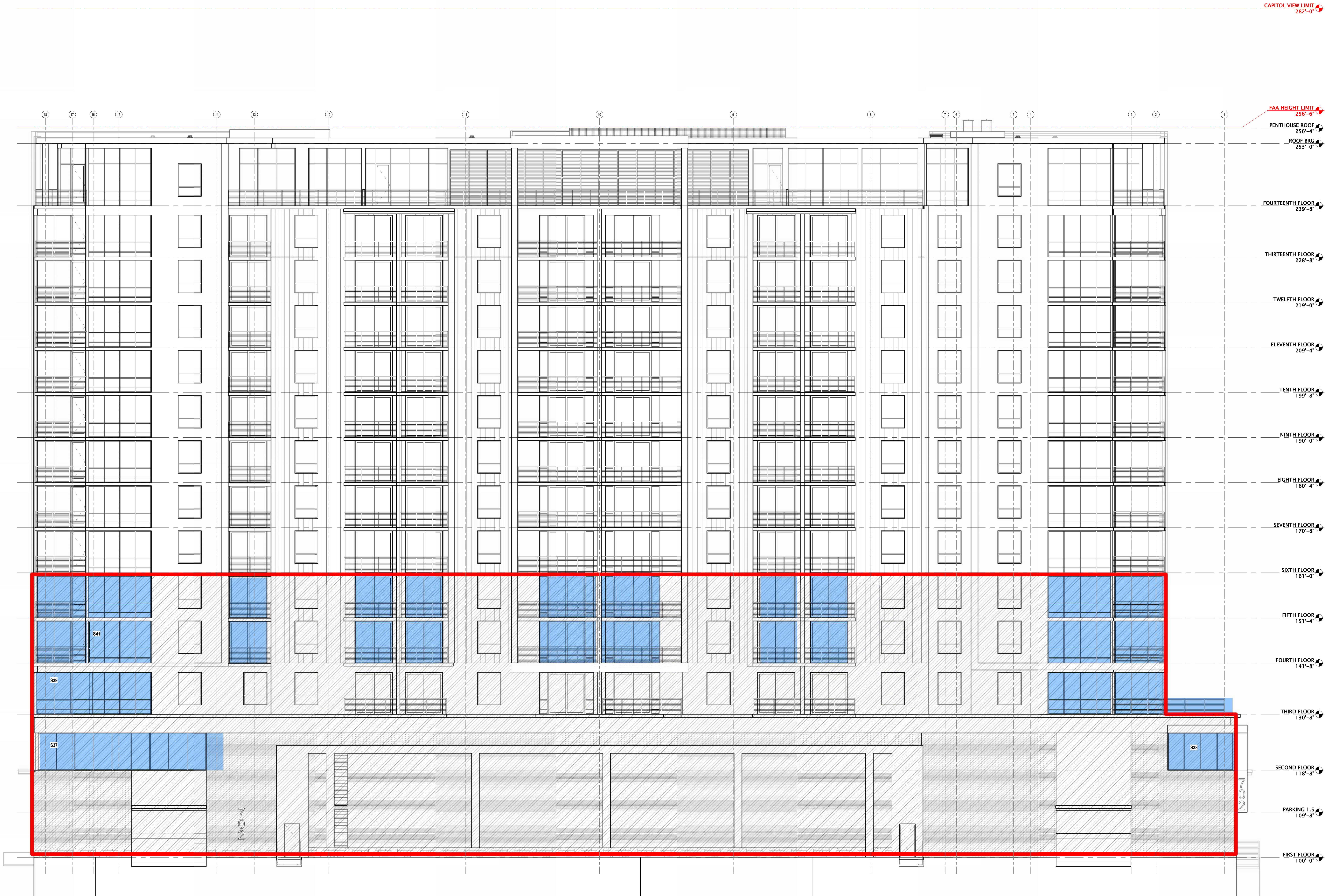
1 NORTH ELEVATION - BIRD SAFE GLASS 1/8" = 1'-0"
