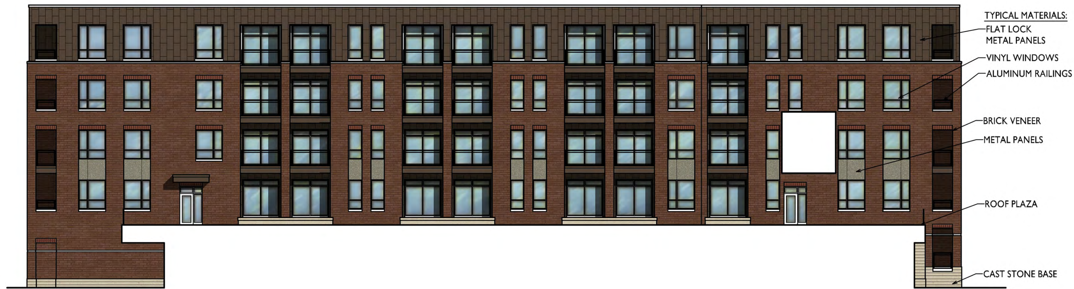
2 COURTYARD ELEVATION A-2.2 1/16"=1'-0"
