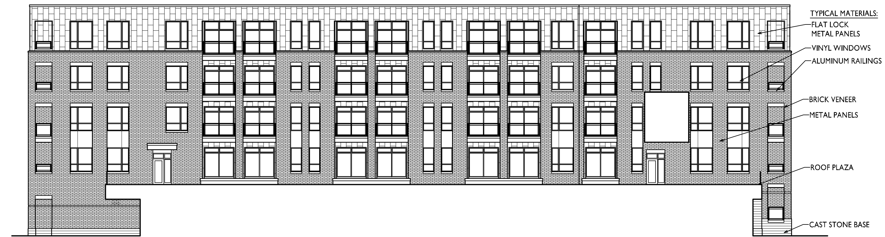
2 COURTYARD ELEVATION A-2.2 1/16"=1'-0"
