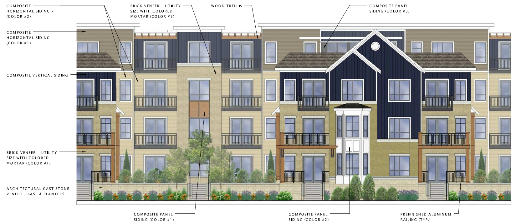
② Mifflin Street Enlarged Elevation - Pitched Roof Option 1/8" = 1'-0"
