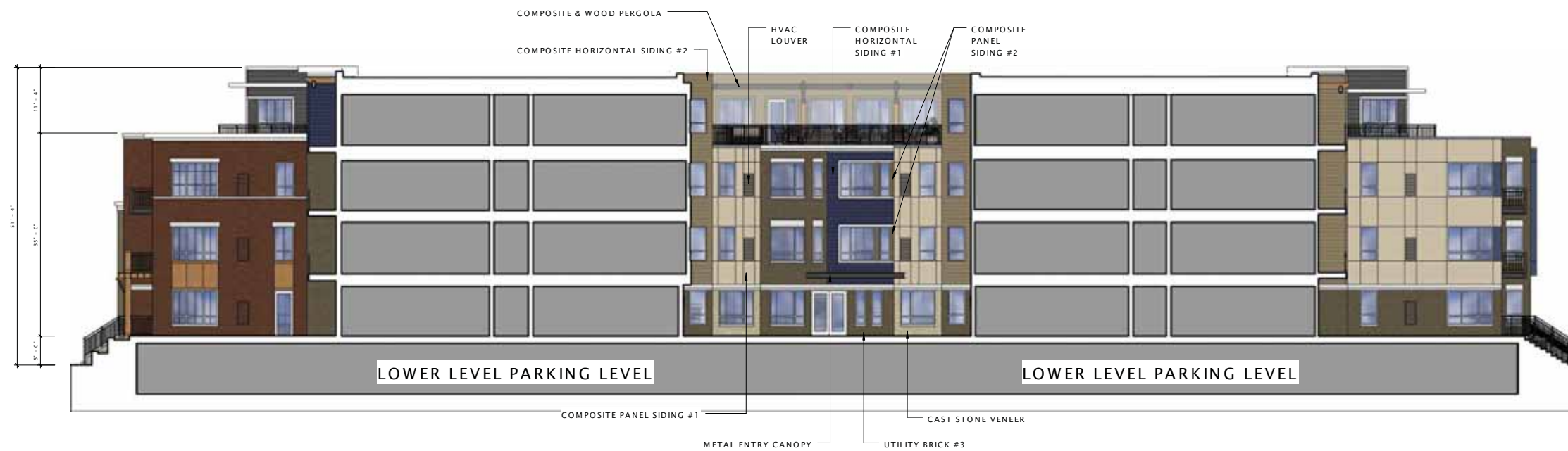
② Interior Courtyard Elevation - North East 3/32" = 1'-0"
