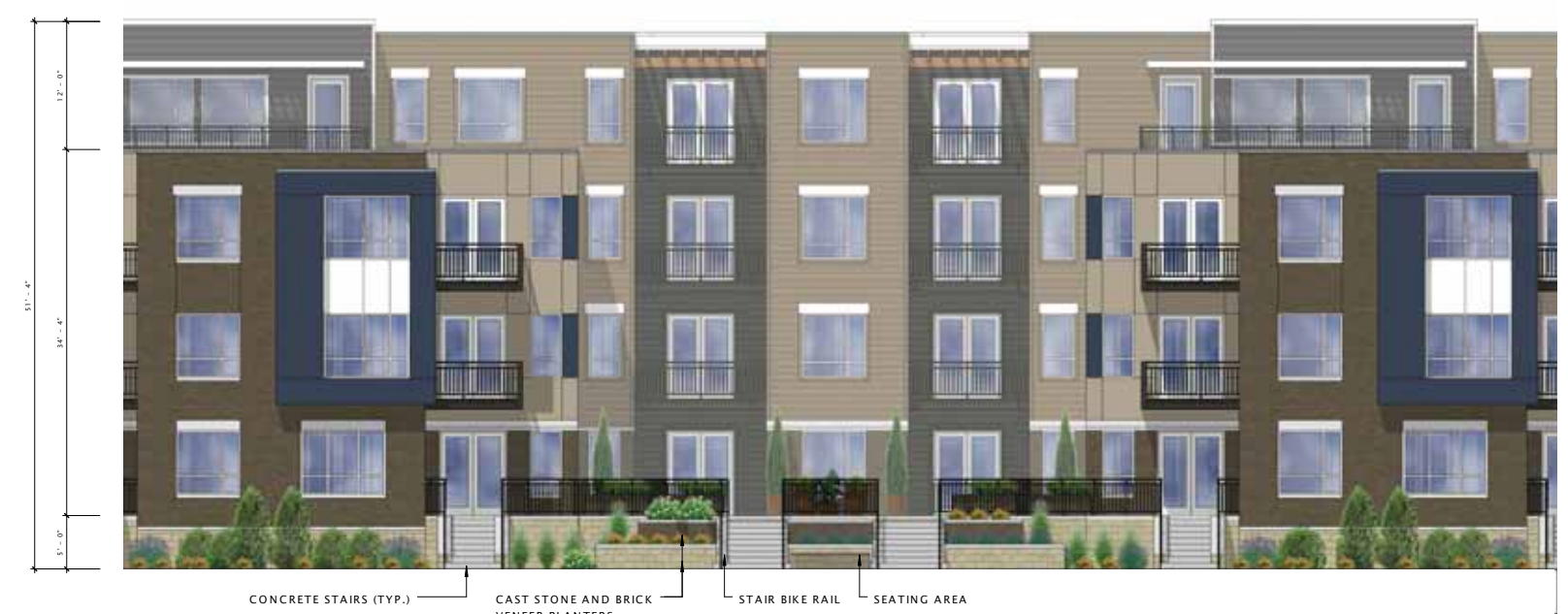
③ Miffin Street Courtyard Enlarged Elevation 1/8" = 1'-0"
