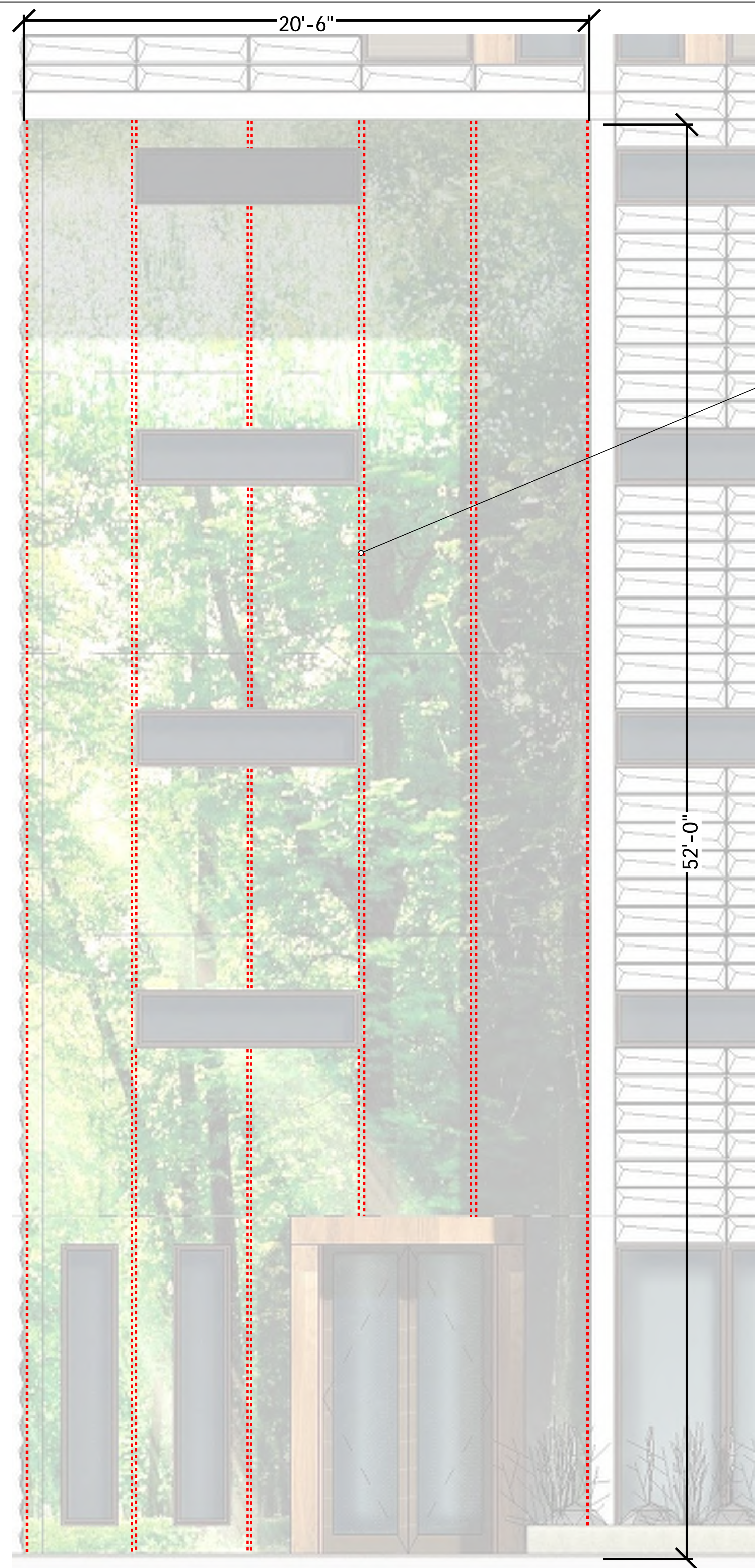
2 North Curtain wall LED light locations
