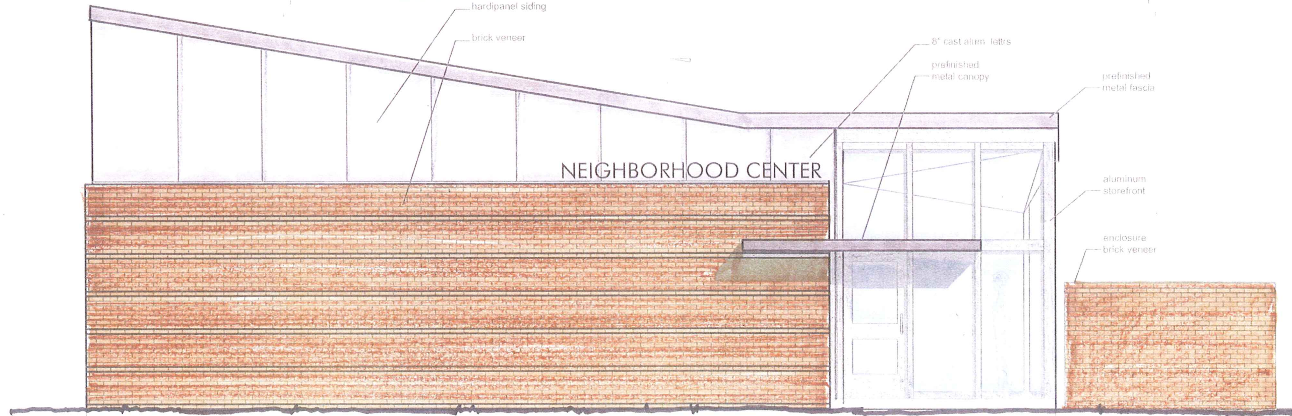
2 South Elevation Scale: 1/2"=1'-0"
