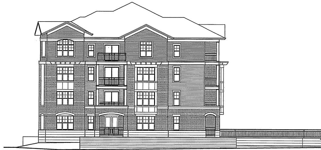
○ END ELEVATION ALONG MAYO DRIVE 3/8" = 1'-0"
