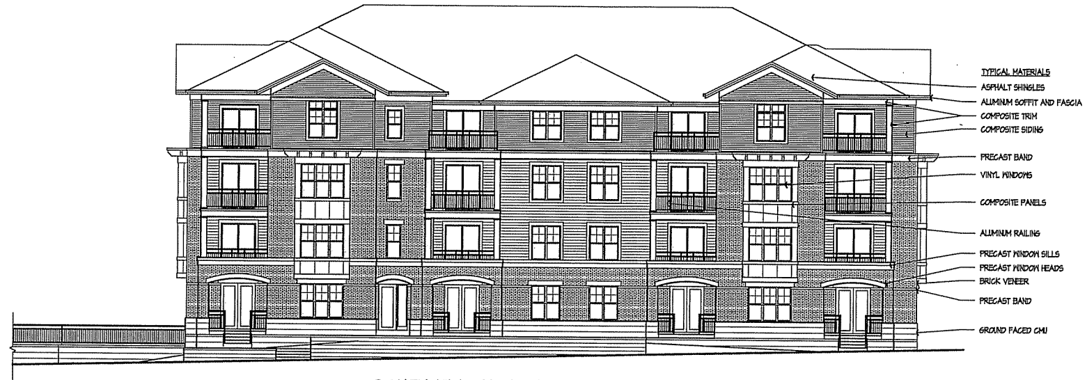
SOUTH ELEVATION ALONG MAYO DRIVE 3/8" = 1'-0"
