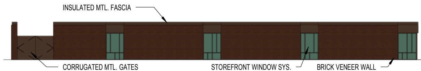
4 TRANSIT HUB - EAST ELEVATION 411 1" = 20'-0"
