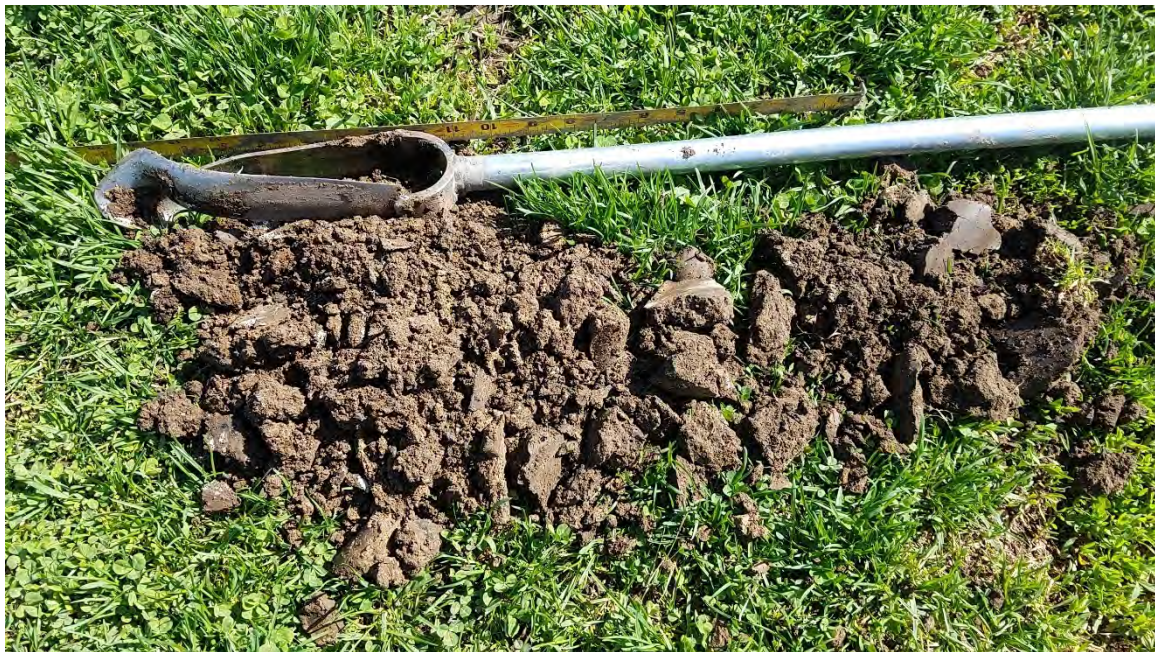
The soils at this sample point appears to be fill material.
