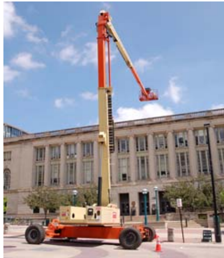
Figure 18 – Boom Lift used for Onsite Survey
