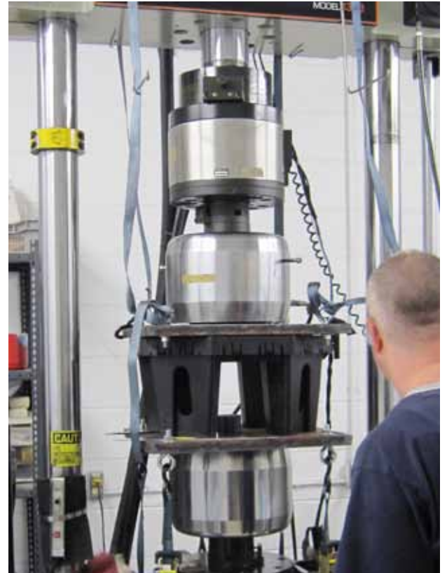
Fig 2.3.12 - Physical load testing of the Strata Cell® GenV.
