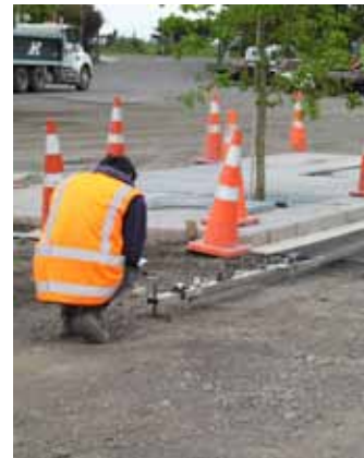
Testing of pavement above and adjacent to structural soil cell treepits. 400 passes on pavement and 200 passes on sidewalk failed to induce any measurable pavement collapse.
