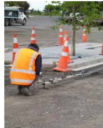
Testing of pavement above and adjacent to structural soil cell treepits. 400 passes on pavement and 200 passes on sidewalk failed to induce any measurable pavement collapse.
