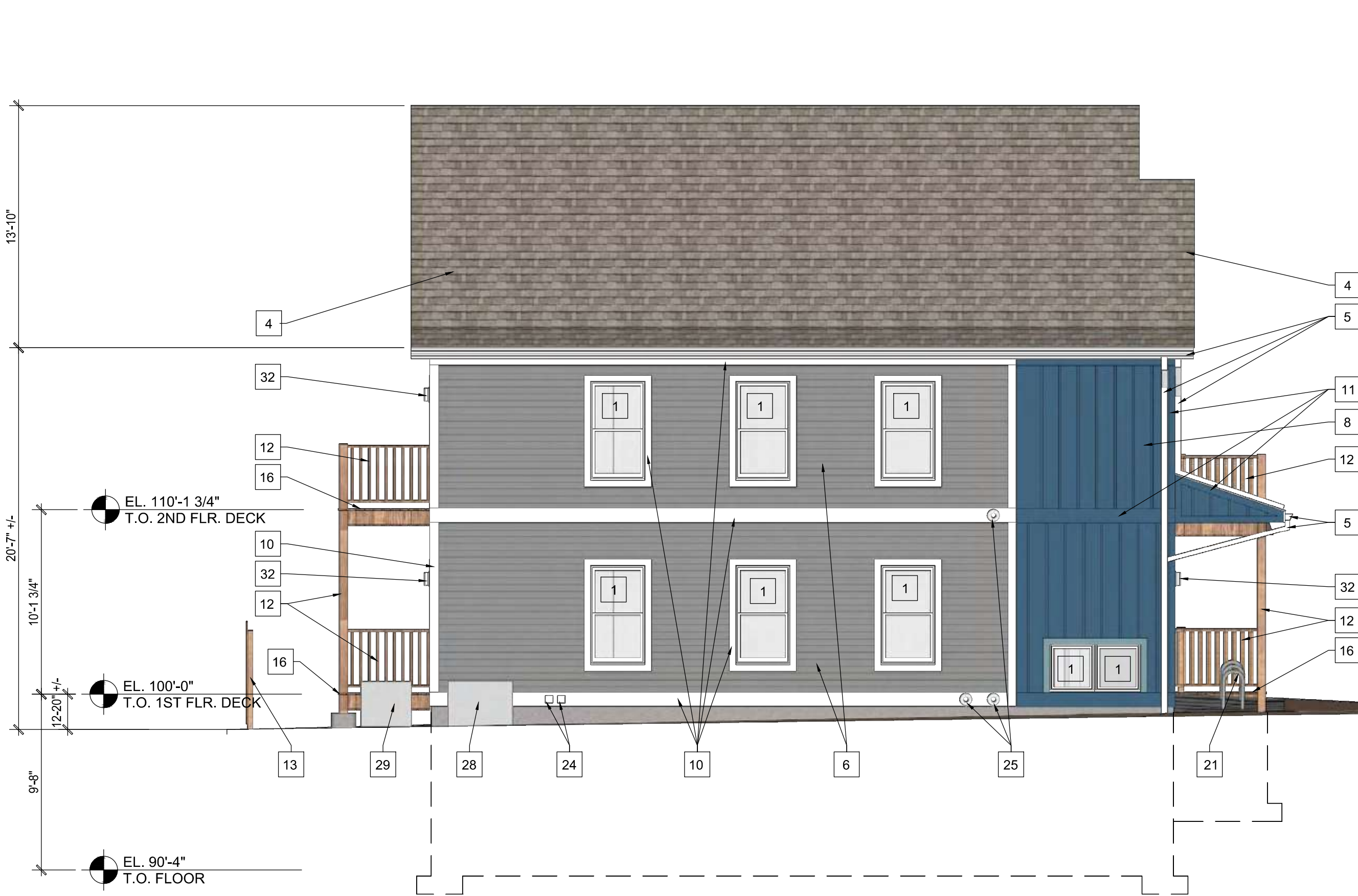
511 W. DAYTON EAST SIDE ELEVATION SCALE: 3/16" = 1'-0"
