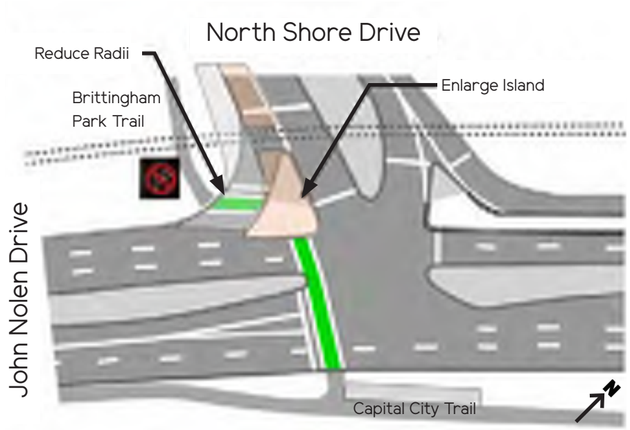
Figure D.15 North Shore Drive-Long Term Solution (Blair Street Corridor Study Report)
