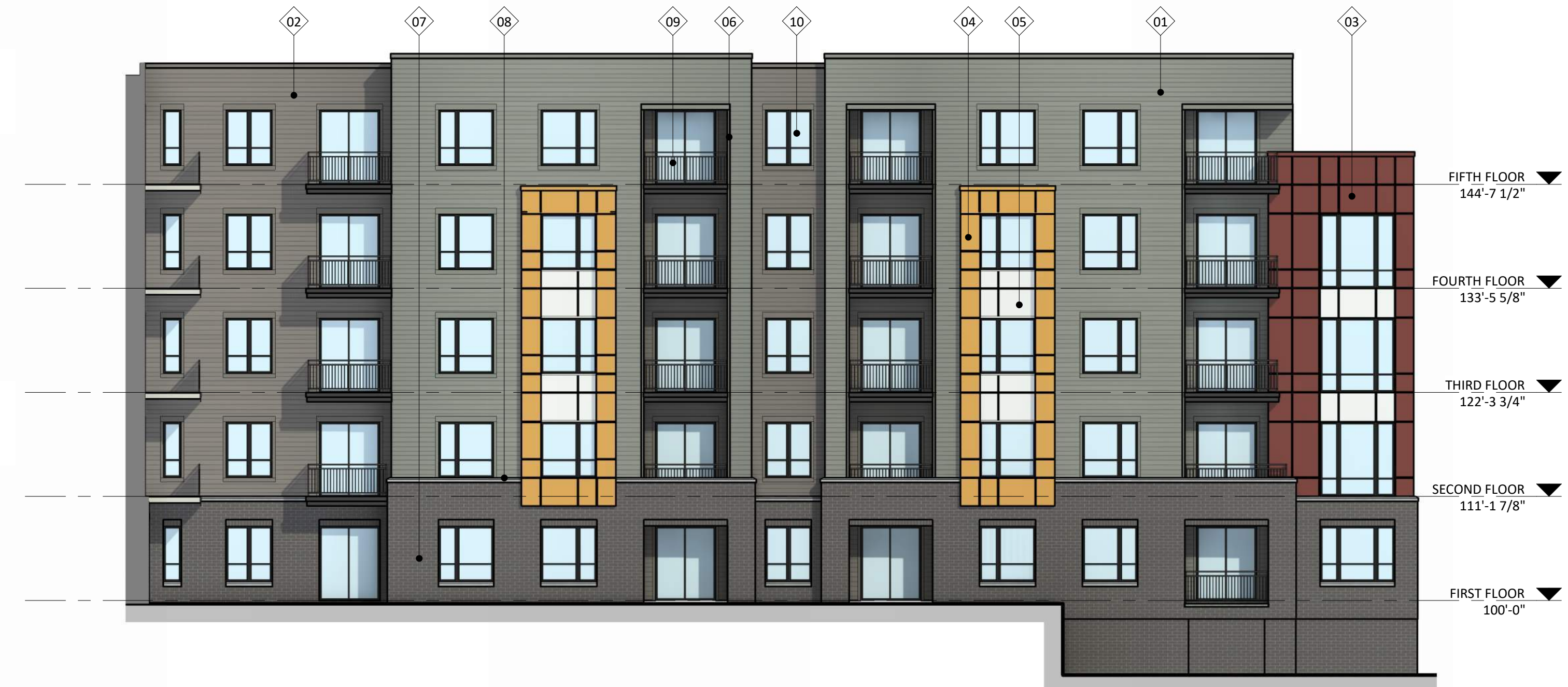
2 COLORED ELEVATION - INTERIOR EAST AC204 3/32" = 1'-0"
