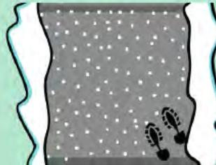
If you apply salt to pavement, aim for a pattern like this, leaving space between salt grains. A coffee mug full of salt is enough for about 60-70 feet of sidewalk. A hand spreader can help create this pattern.
