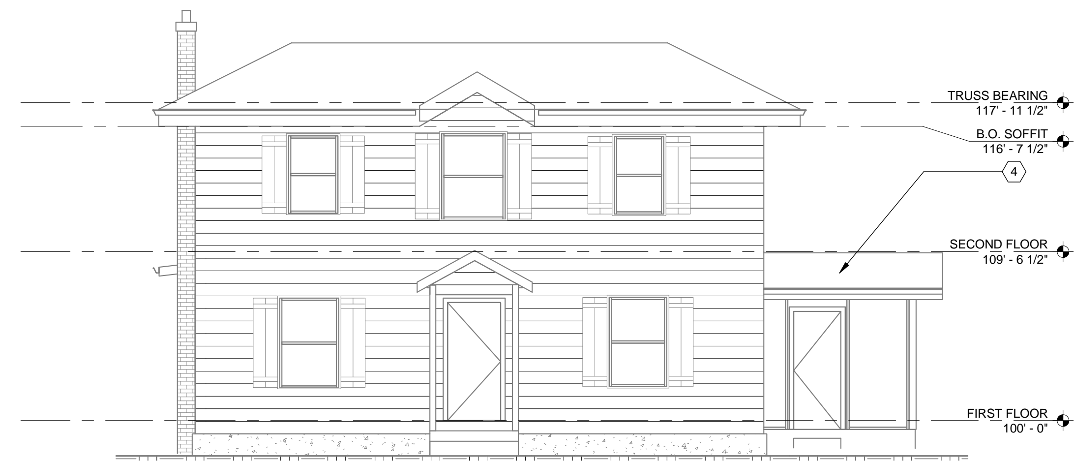
4 SOUTH ELEVATION - NEW WORK 3/16" = 1'-0"
