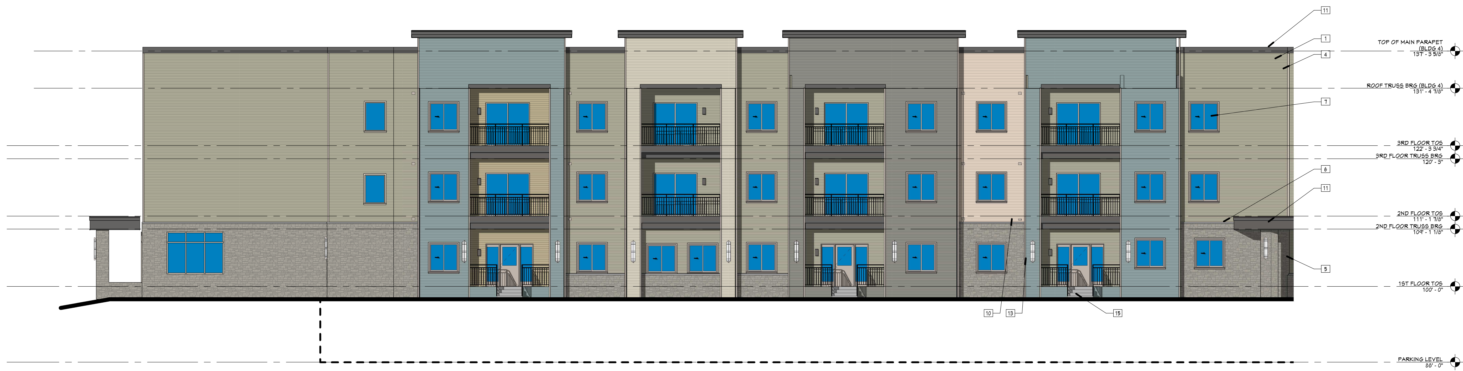
1 SOUTHWEST ELEVATION - BUILDING 4 - ZONE G A4.7 1/8" = 1'-0"
