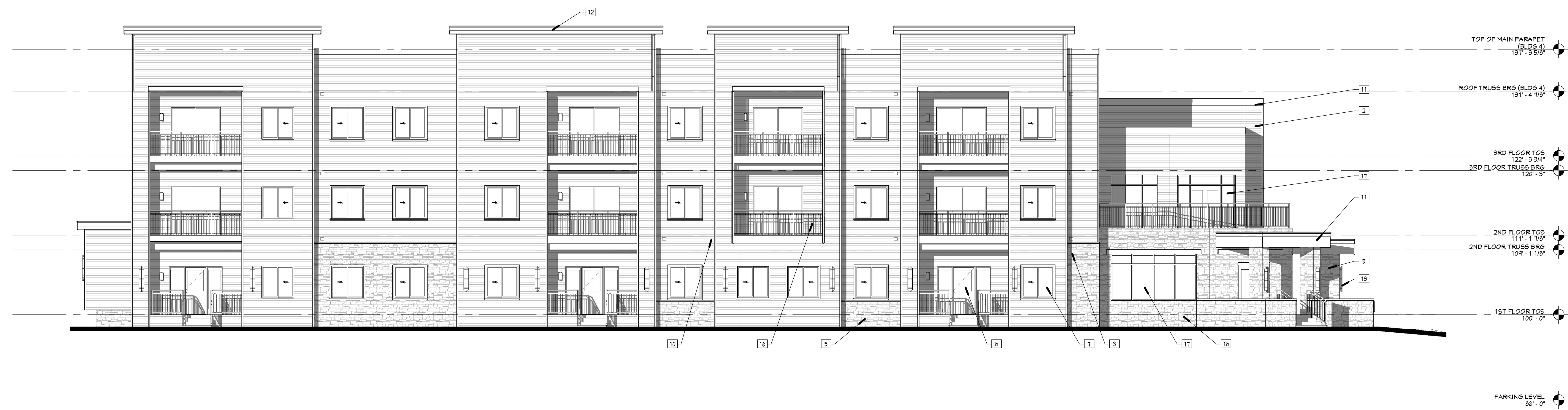
1 SOUTH ELEVATION - BUILDING 4 - ZONE F A4.6 1/8" = 1'-0"
