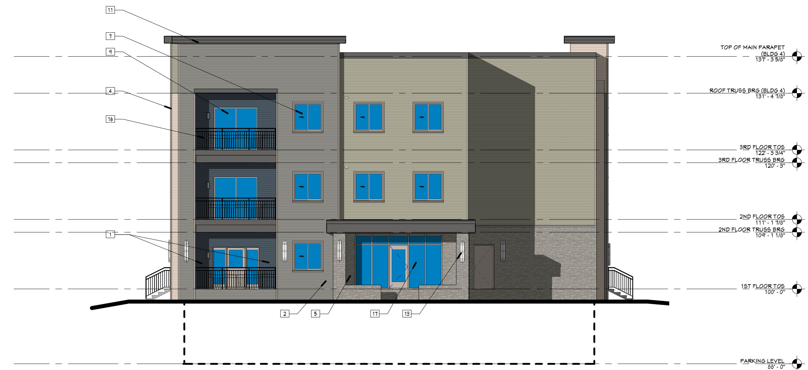
2 NORTHWEST ELEVATION - BUILDING 4 - ZONE G A4.7 1/8" = 1'-0"
