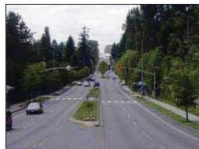
FIGURE 4.19 Wide boulevards can be aesthetically pleasing and can act as a pedestrian refuge for those trying to cross the street
