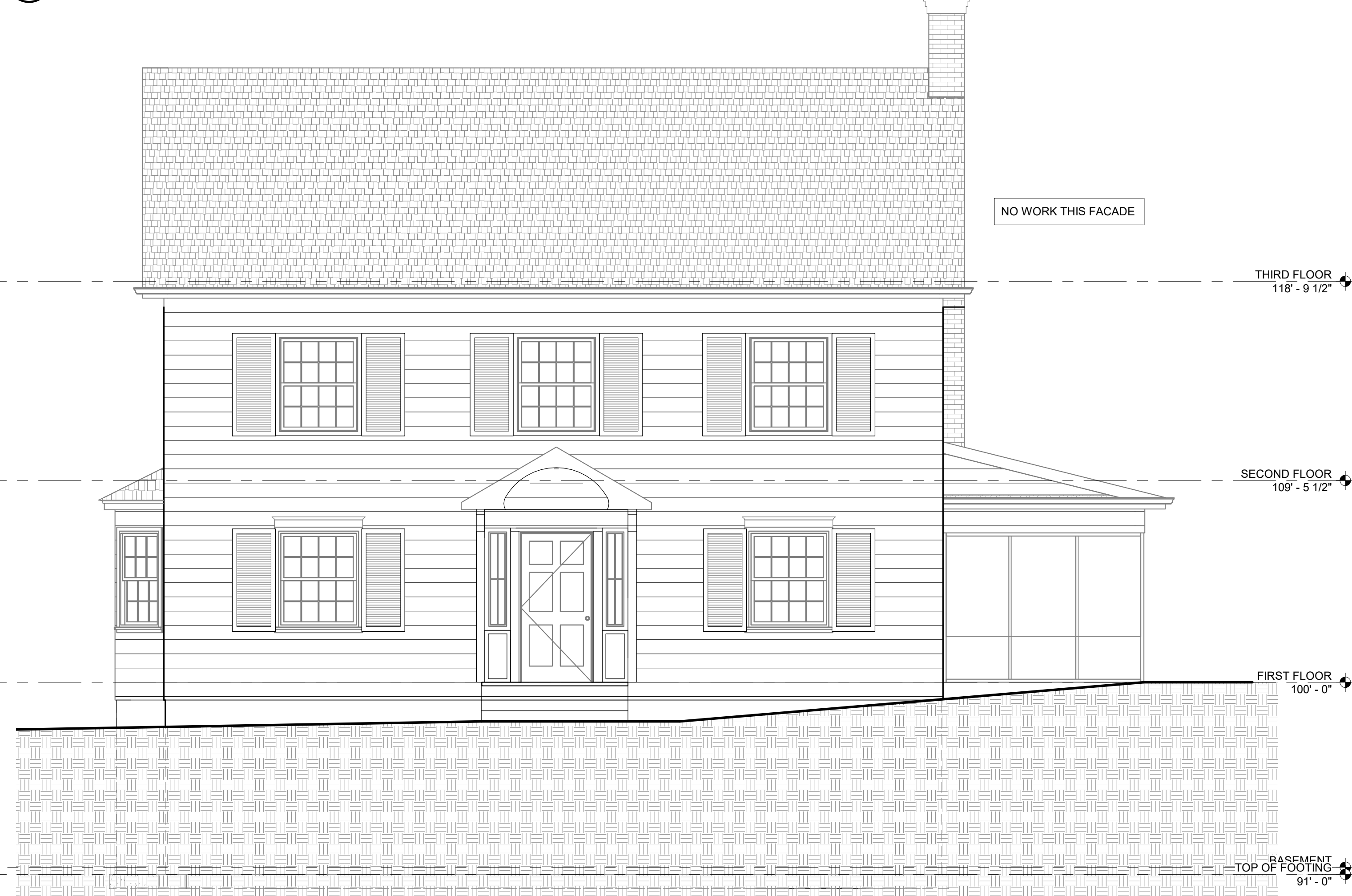
1 SOUTH ELEVATION - HOUSE 1/4" = 1'-0"
