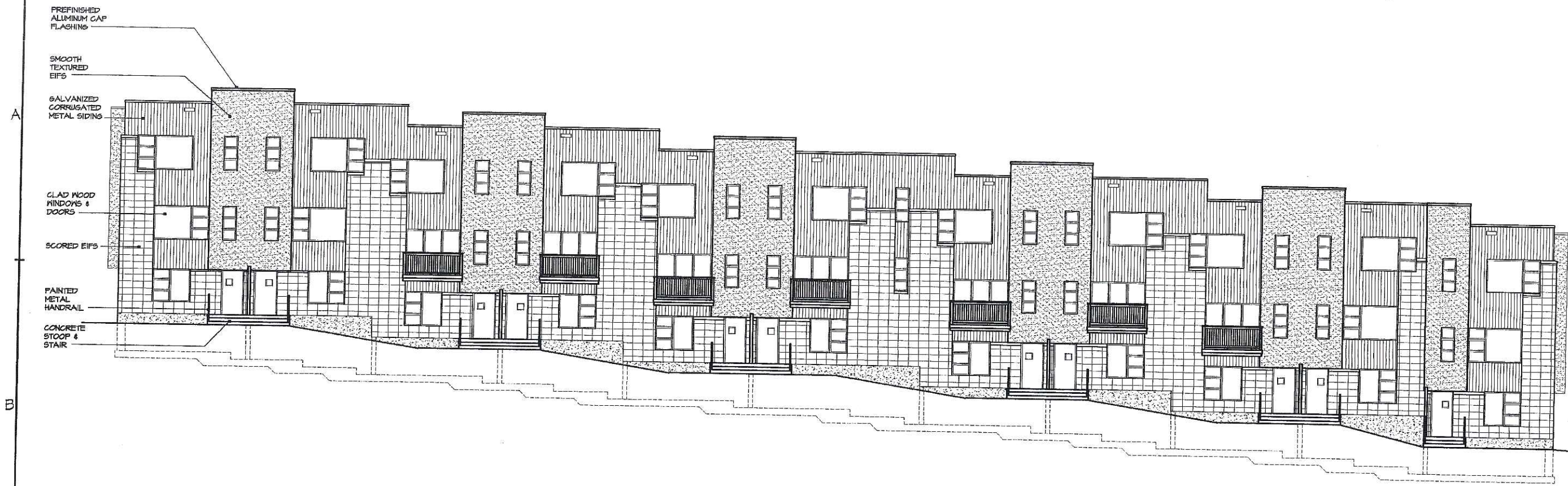
(A) 12 UNIT COMPOSITE FRONT ELEVATION SCALE: 1/8" = 1'-0"
