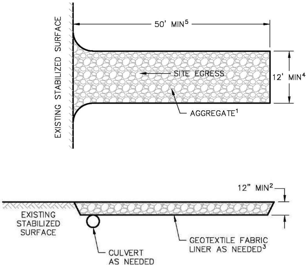
Note 1 Use hard, durable, angular stone or recycled concrete meeting the gradation in Table 1. Where this gradation is not available, meet the gradation in Wisconsin Department of Transportation (DOT) 2018 Standard Specification, Section 312, Select Crushed Material.
