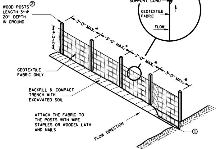
\* NOTE: 8'-0" POST SPACING ALLOWED IF A WOVEN GEOTEXTILE FABRIC IS USED.
