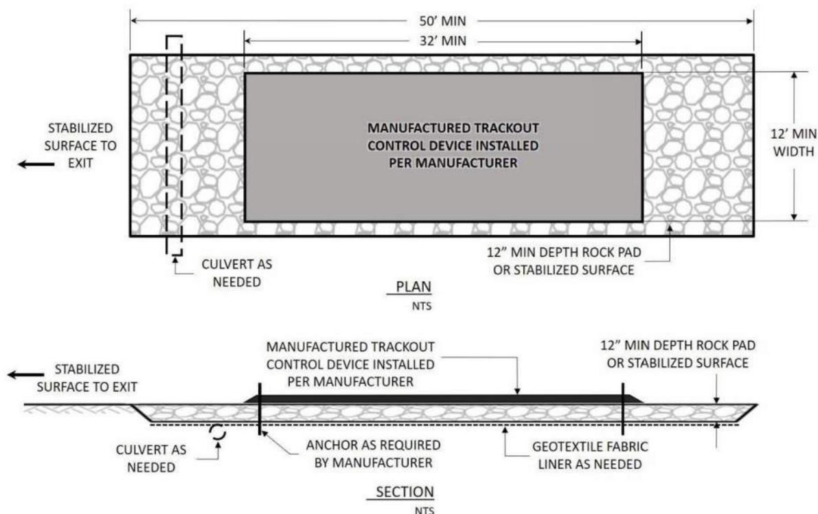
Note 1 This detail is provided as an example. Comply with manufacturer’s specifications while also meeting the minimum manufactured tracking pad length and width described in this technical standard.
