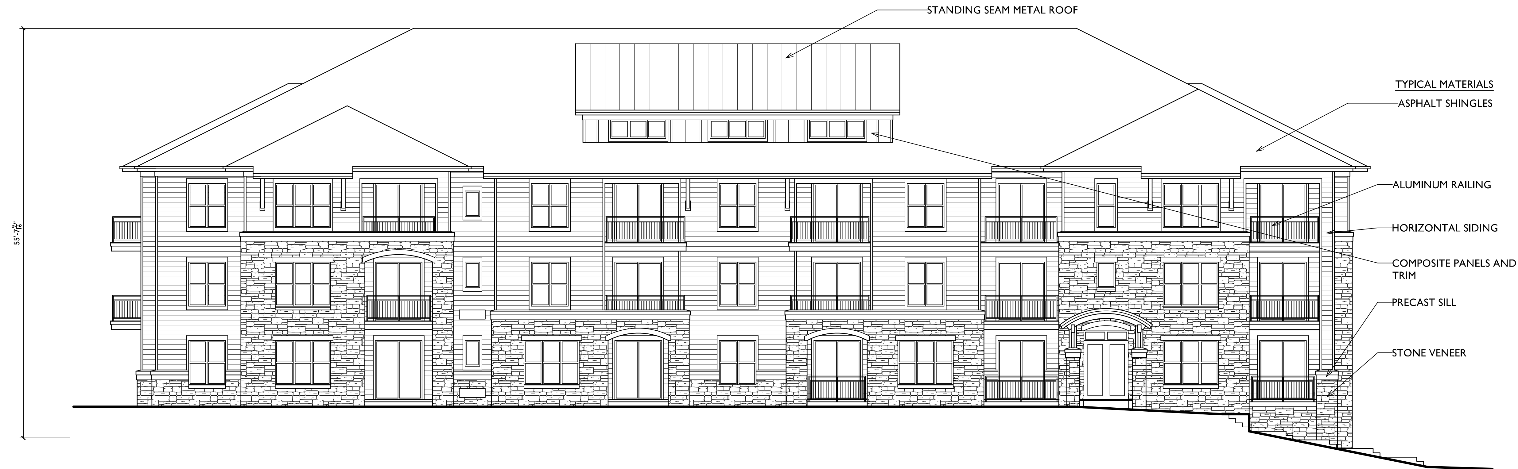
1 21 NORTH ELEVATION - BUILDING 4 SCALE: 1/8"=1'-0"
