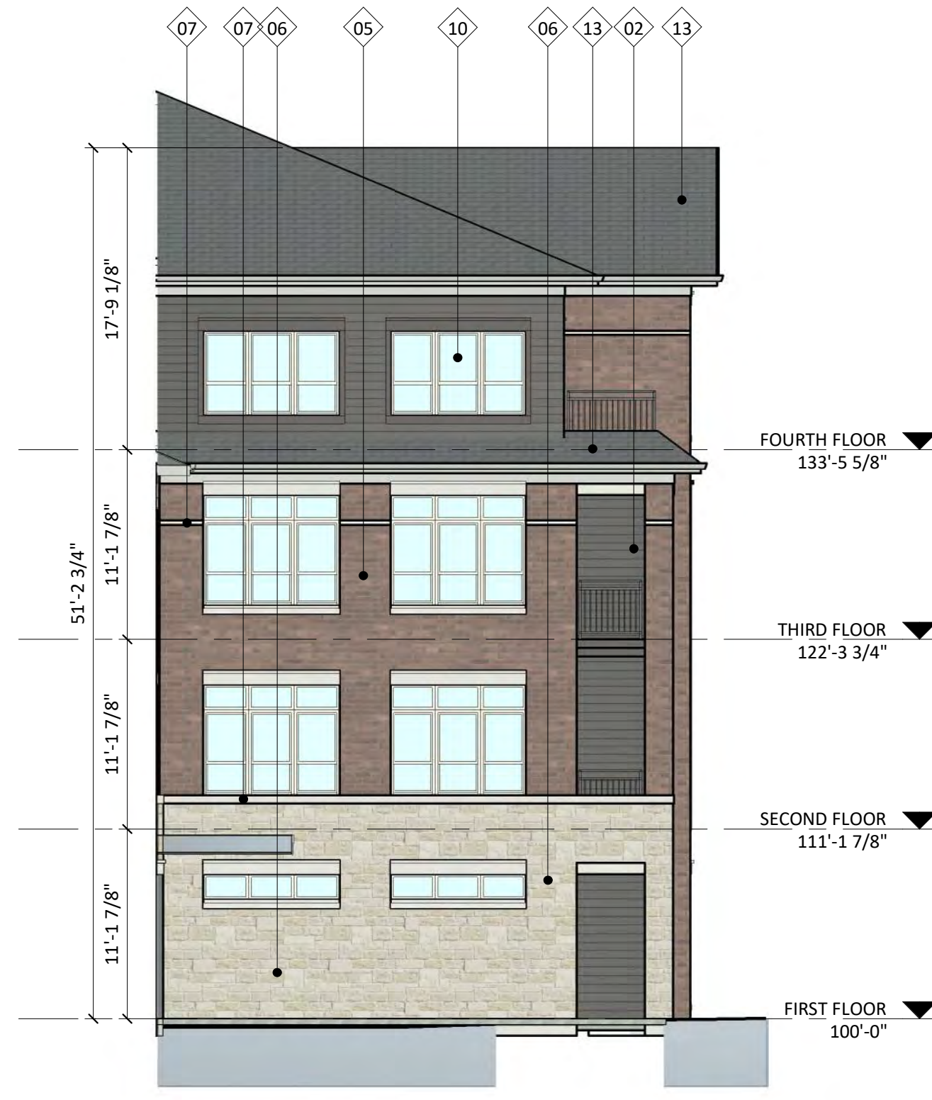
4 COLORED ELEVATION - A - ENTRY CORRIDOR 1.2 A-2.13 1/8" = 1'-0"
