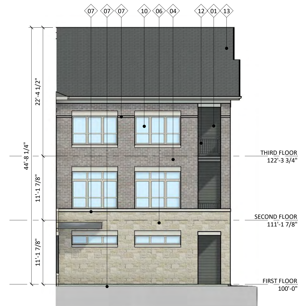
2 COLORED ELEVATION - C - ENTRY CORRIDOR 1.2 A-2.20 1/8" = 1'-0"
