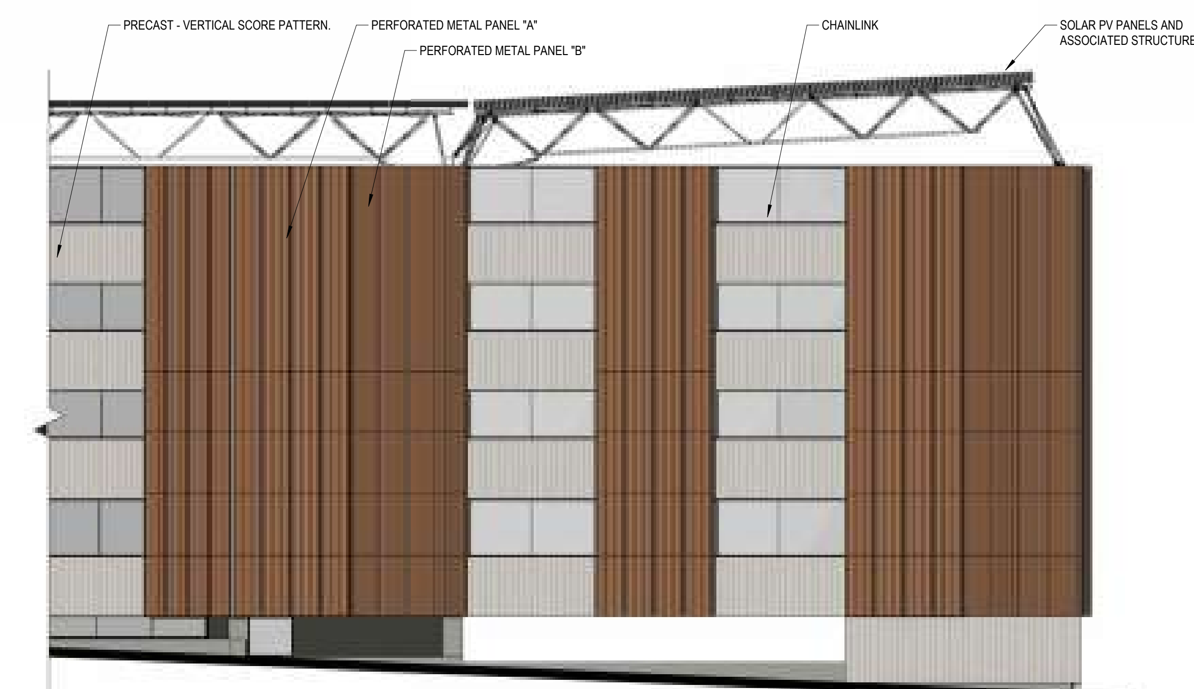
B6 PARKING NORTH ELEVATION 1" = 10'-0"
