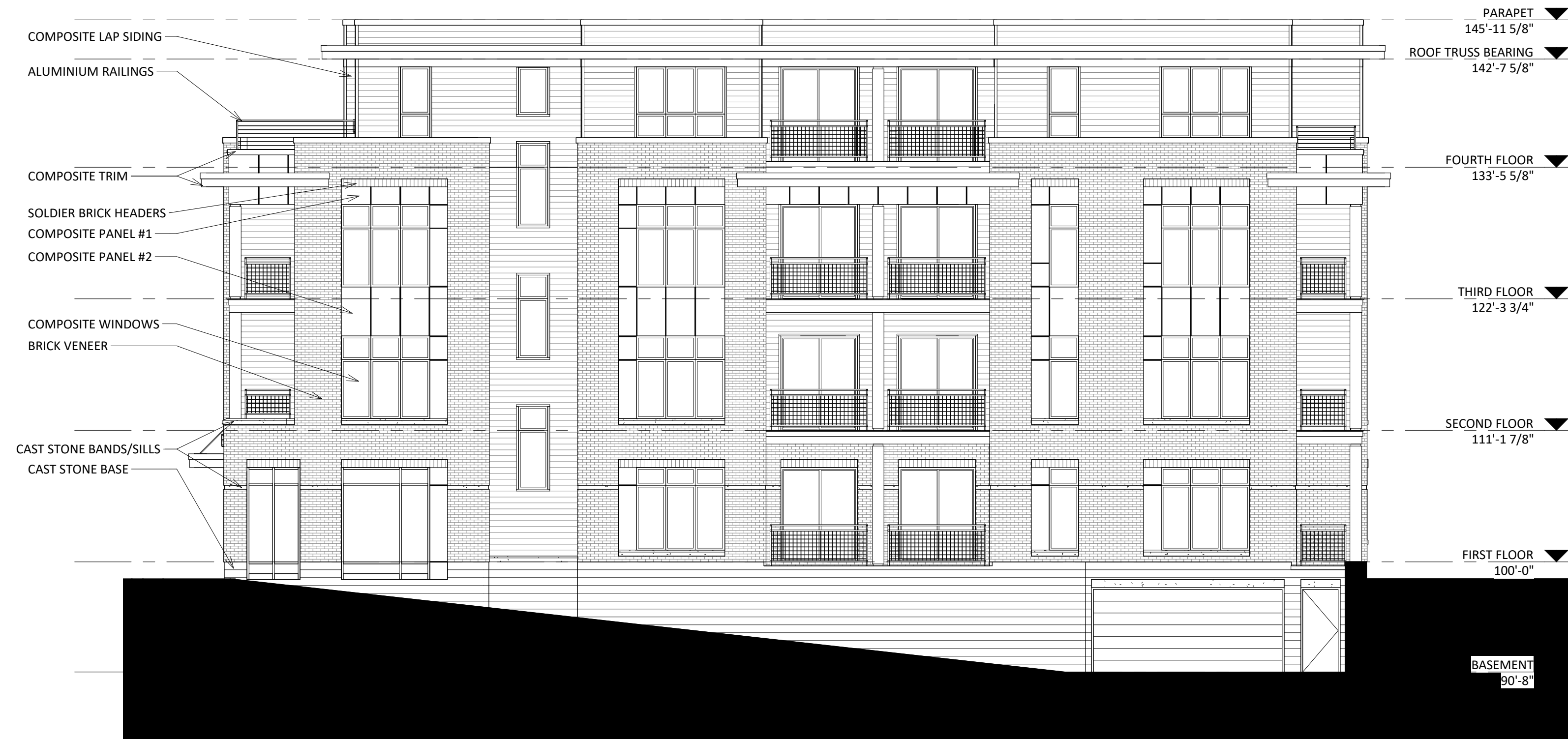
2 ELEVATION - NORTH A-2.1 1/8" = 1'-0"
