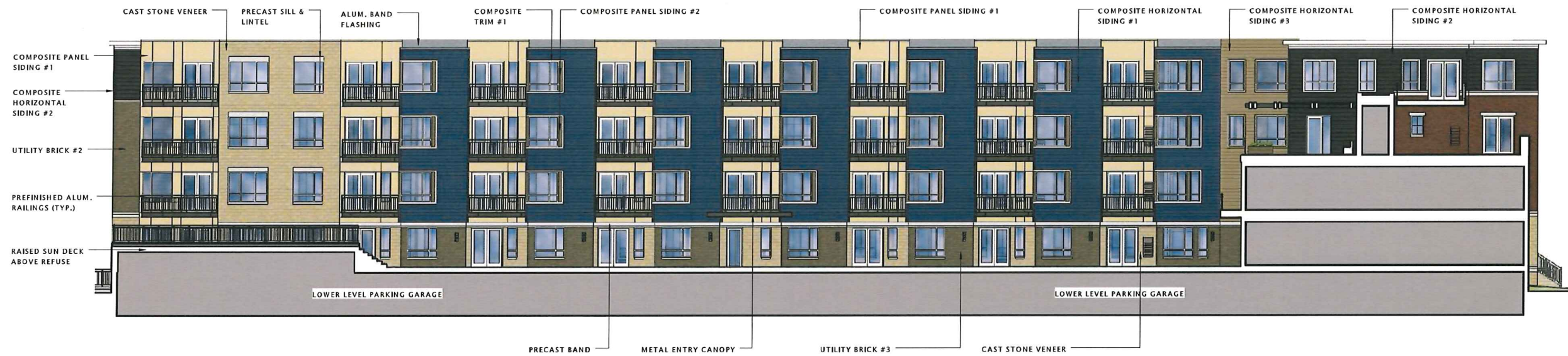
② Interior Courtyard Elevation - South 3/32" = 1'-0"
