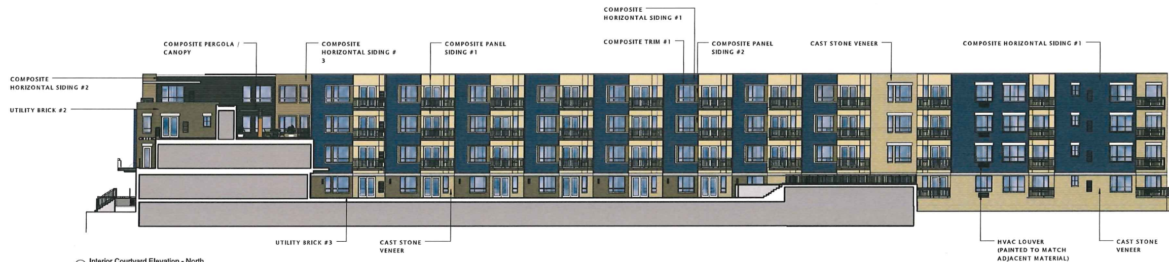
③ Interior Courtyard Elevation - North 1/16" = 1'-0"
