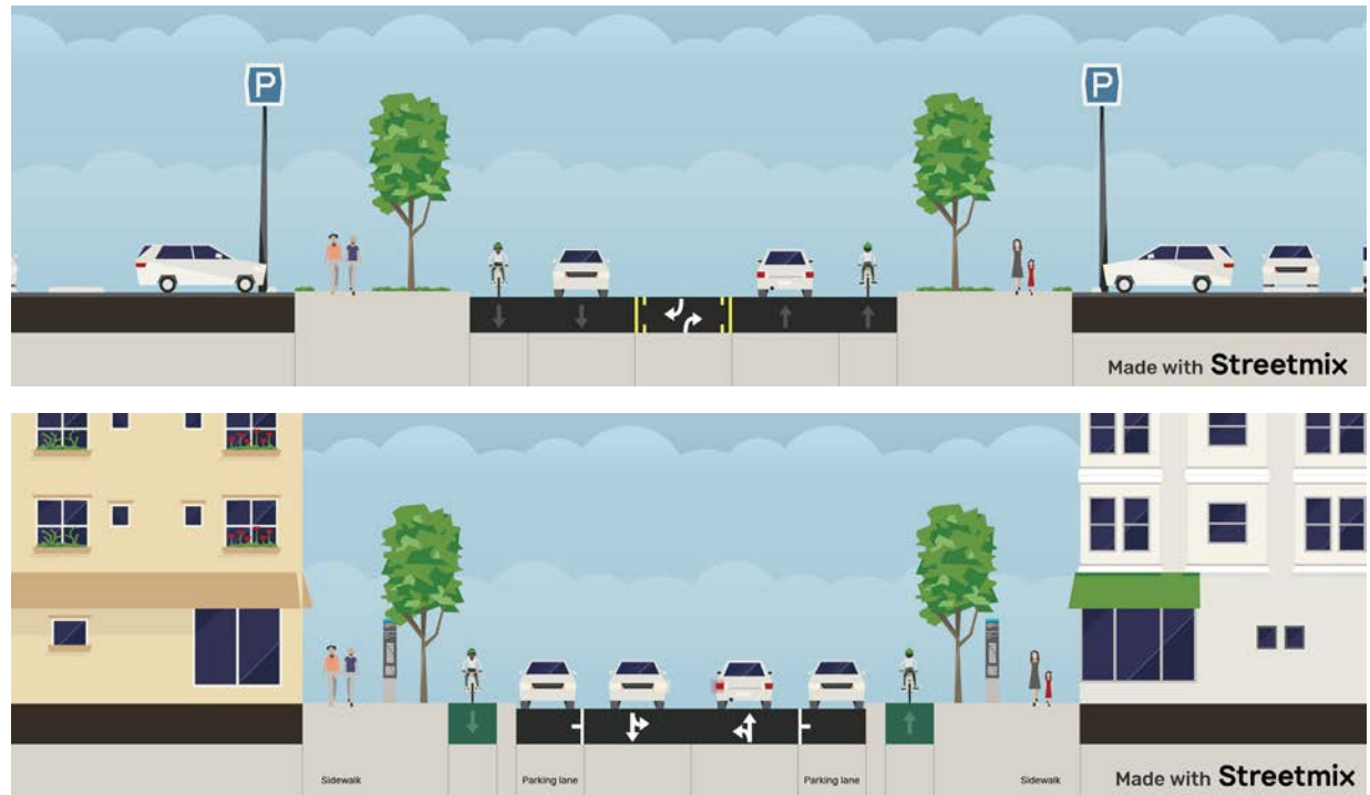
Cross-sections show existing East Towne Boulevard (top). With redevelopment over time, East Towne Boulevard should feature protected bike lanes, on street parking, and at least six foot sidewalks.
