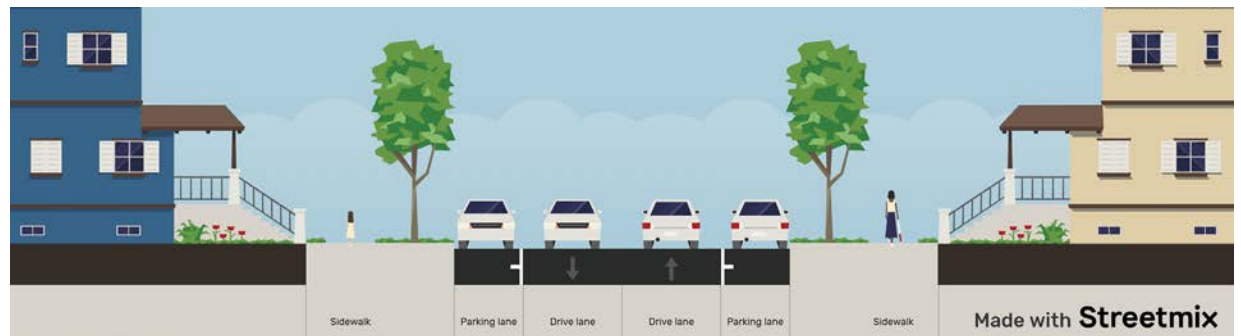
Street cross-section of a new local street surrounded by smaller-scale housing within the area designated for Low-Medium Residential
