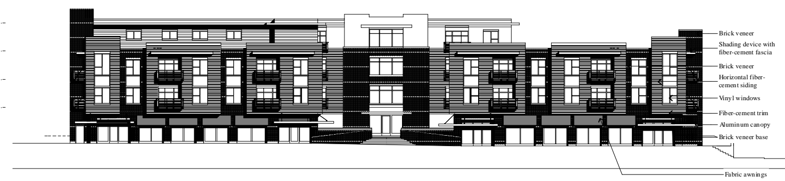
South Elevation - Phase II
