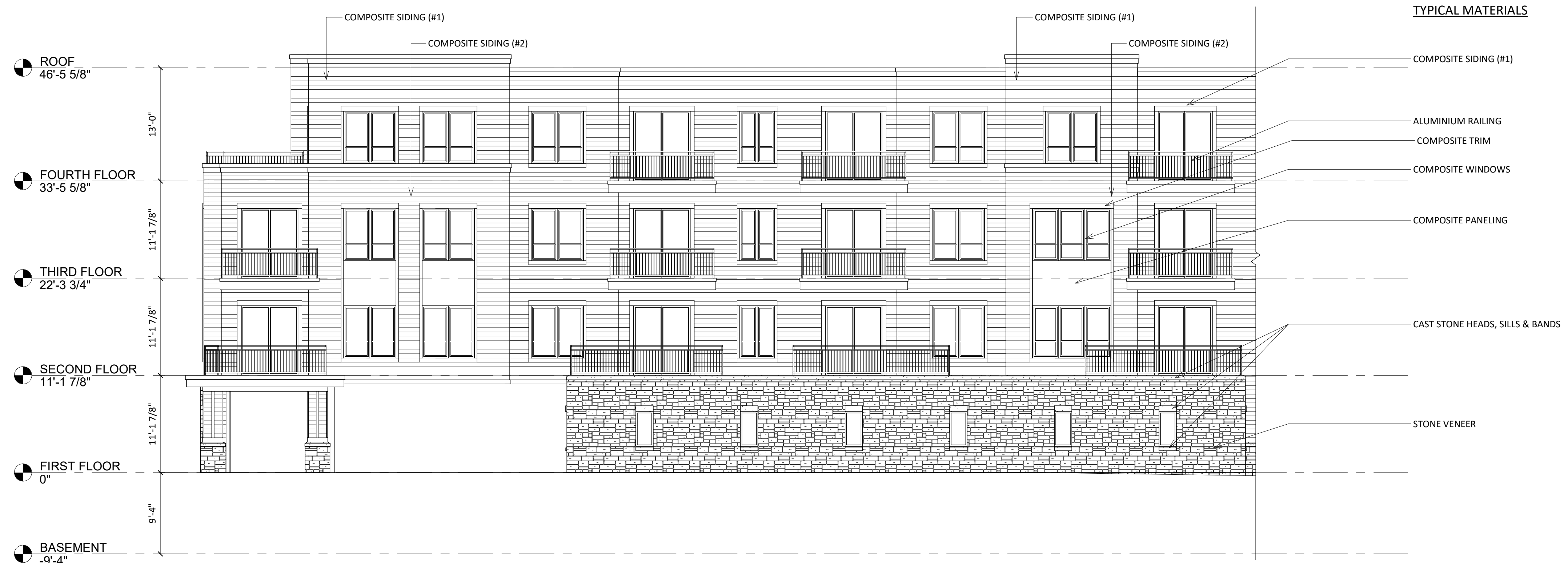
2 PARTIAL EAST ELEVATION A-2.3 1/8" = 1'-0"
