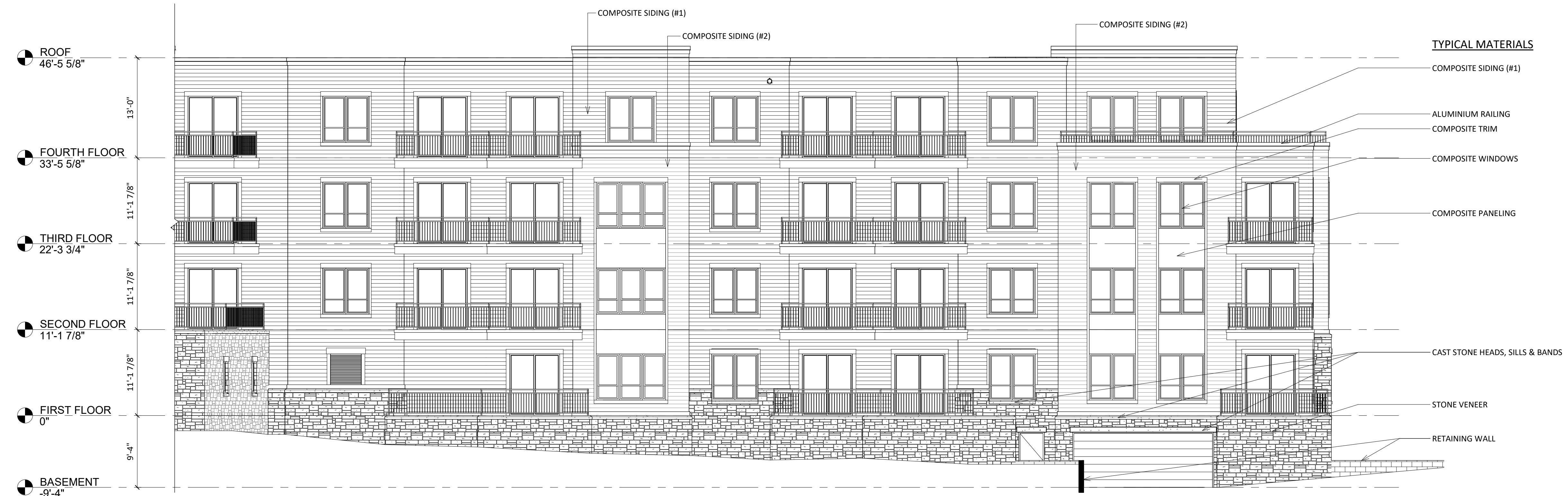
1 PARTIAL EAST ELEVATION A-2.3 1/8" = 1'-0"
