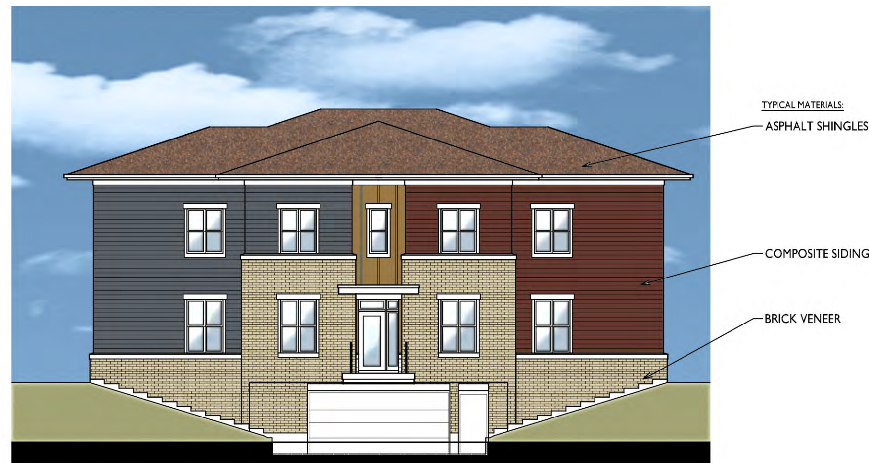
2 WEST ELEVATION A-2.1 3/32"=1'-0"
