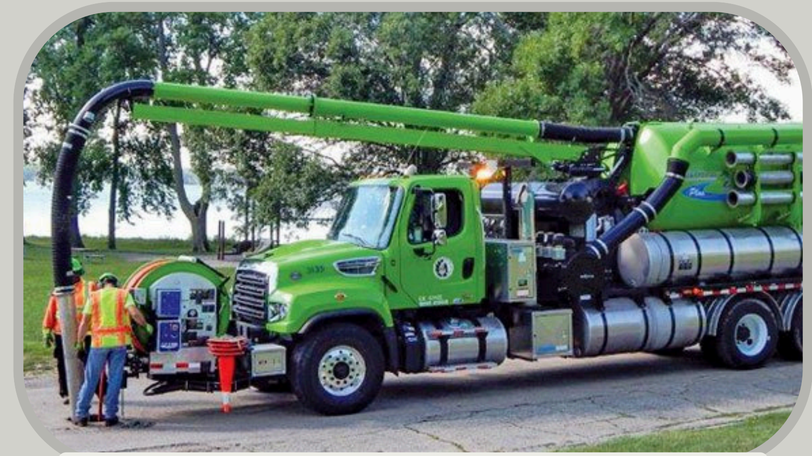
Vactor Truck used to clean sewer and address emergency back-ups
