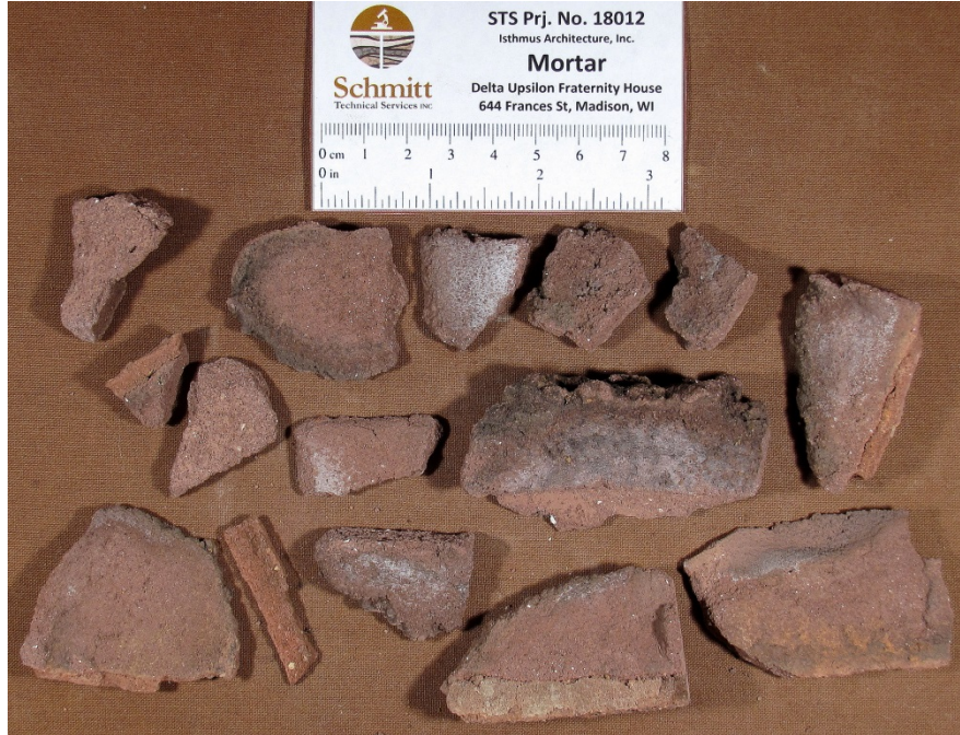
Photograph 1. Unlabeled mortar sample in the condition received for testing. Top scale is in centimeters. Bottom scale is in inches.
